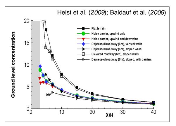
Wind tunnel simulations show roadway design effects on pollutant transport and dispersion. Highest levels occur with at-grade and elevated fill roads. Lowest levels occur with cut sections and noise barriers
