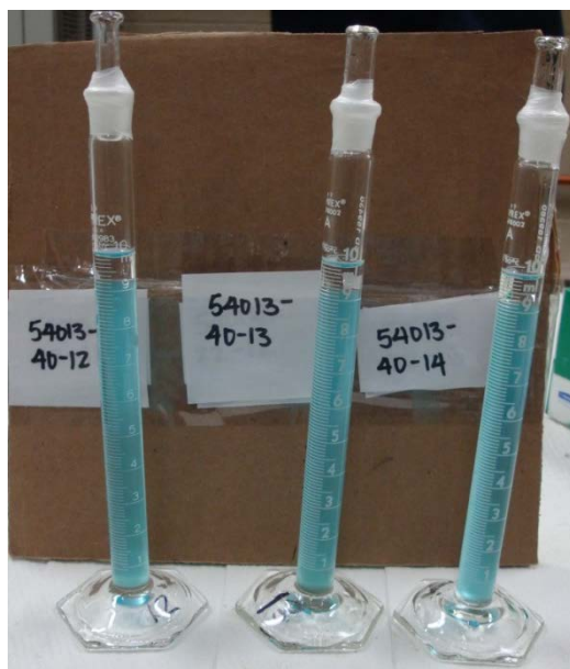
Figure 5. Photo taken during Non-Additive Volume Experiment for E85. The test was completed in triplicate. This particular photo occurred after the last water addition. The water was dyed with blue food coloring.
