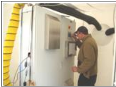
Figure 4 VHP generation system.
