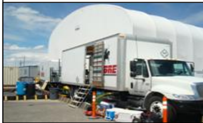
Figure 6. Truck-mounted gas-generation system.
