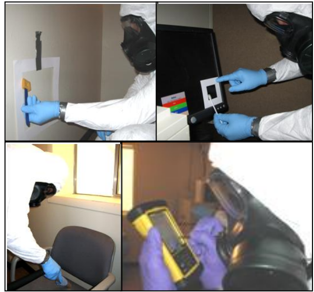
Figure 7. Above: Wipe sampling: sponge-stick and swab. Below: Vacuum sampling (left) and PDA with BROOM software (right).
