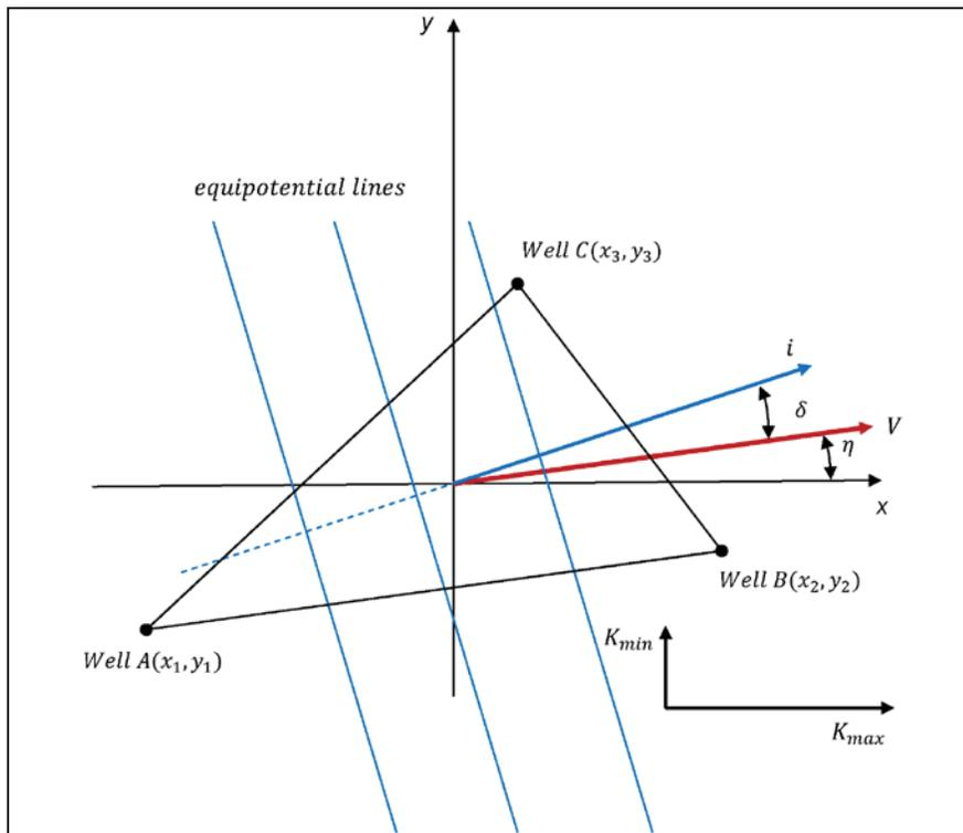
Figure A-5. Terminology used in this derivation of the direction of the groundwater velocity vector in an anisotropic medium. The hydraulic gradient vector is the blue arrow labeled  $i$  and the groundwater velocity vector is the red arrow labeled  $V$ .
