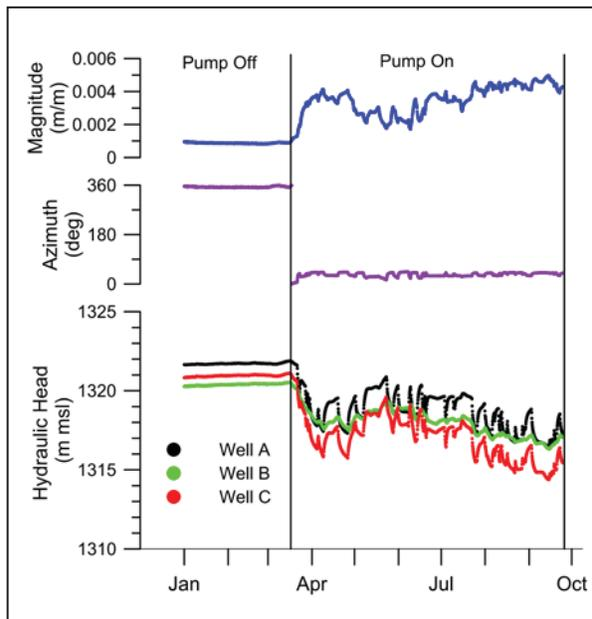
Figure 11. Hydraulic heads measured using pressure transducers in wells A, B, and C and the resulting magnitude and direction (azimuth) of the hydraulic gradient measured in degrees from North. When the irrigation well is not pumping, the hydraulic gradient is low and oriented approximately north. During the agricultural season, the hydraulic gradient increases in magnitude and the orientation shifts to the northeast toward the irrigation well.
