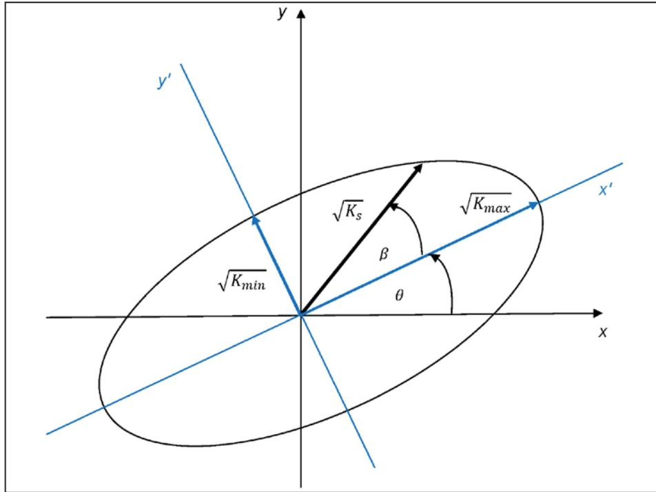
Figure A-4. Terminology used in calculation of the hydraulic conductivity ellipsoid including the major semi-axes oriented in the directions of the maximum and minimum hydraulic conductivity. The hydraulic conductivity  $K_s$  in any direction of flow in an anisotropic aquifer can be determined graphically or using Equation (A-20).
