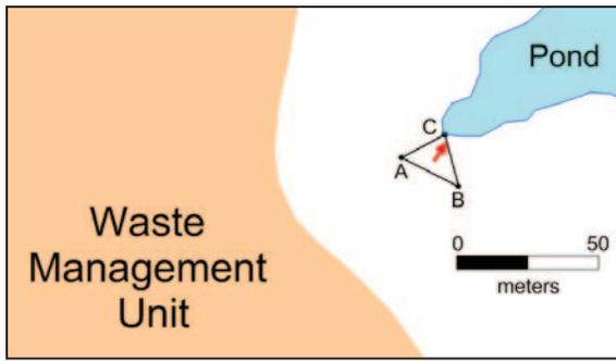
Figure 12. Site map depicting triangle of wells used to estimate hydraulic gradients. The average hydraulic gradient vector (red arrow) indicated groundwater flow was to the pond during the monitoring period.
