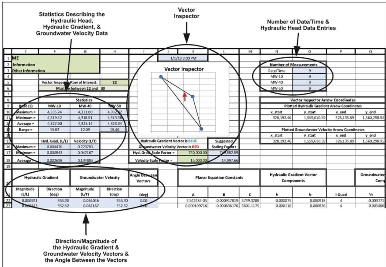
Figure 3. Screen capture from the 3PE spreadsheet depicting results of the hydraulic gradient and groundwater velocity vector calculations and the Vector Inspector feature. Cells for user input are shaded green. Blue cells are the most significant results of the calculations.
