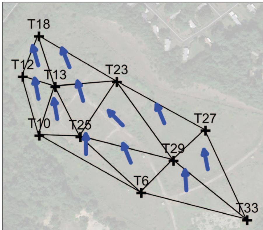
Figure 16. Network of three-point problems used to calculate hydraulic gradients and the resulting average (net) direction of the hydraulic gradient within each triangle (blue arrows). The monitoring wells (crosses), three-point solution triangles, and output vectors from the 3PE spreadsheet were plotted on a georeferenced base map to enhance conceptualization of groundwater flow directions across the site.
