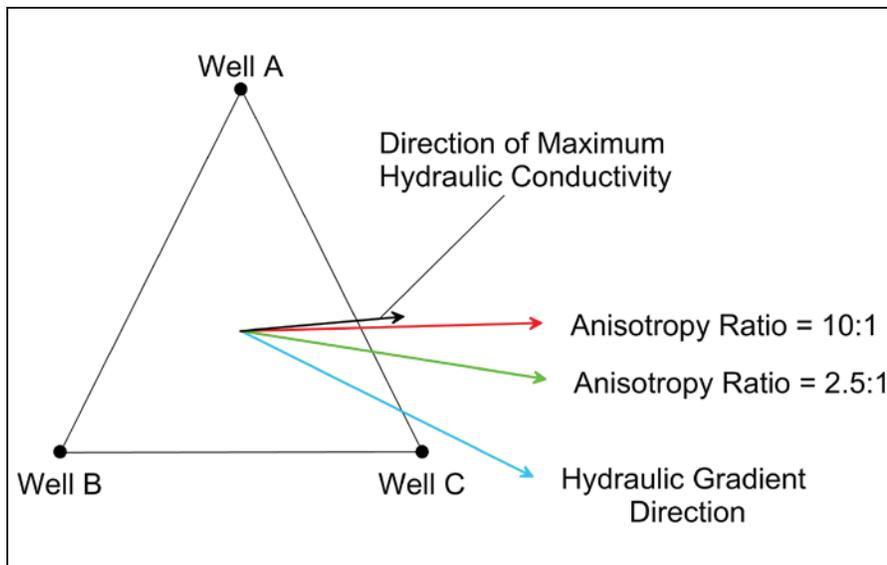
Figure 17. Effects of anisotropy in horizontal hydraulic conductivity on groundwater flow directions. The blue arrow (direction of the hydraulic gradient) would be the direction of groundwater flow in an isotropic setting. In a situation with horizontal anisotropy, the direction of groundwater flow shifts toward the direction of the maximum hydraulic conductivity as the ratio  $K_{max}:K_{min}$  increases.
