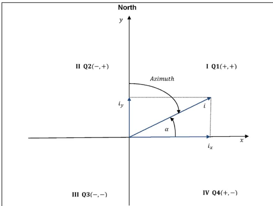
Figure A-2. Definition of the quadrants and vector angles used in this derivation. Note that the mathematical convention used to number the quadrants in the derivation proceeds in a counter-clockwise direction from the positive  $x$ -axis. In the 3PE spreadsheet, the familiar geological convention in which the quadrants are numbered in a clockwise fashion starting at the positive  $y$ -axis (North) was implemented.
