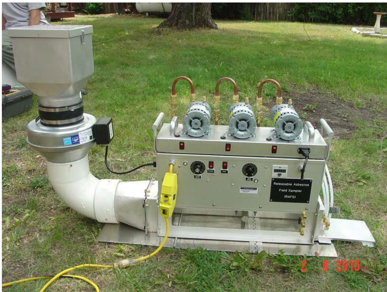
Figure 8. Aluminum (or equivalent non-porous surface) for collection quality assurance equipment blank.
