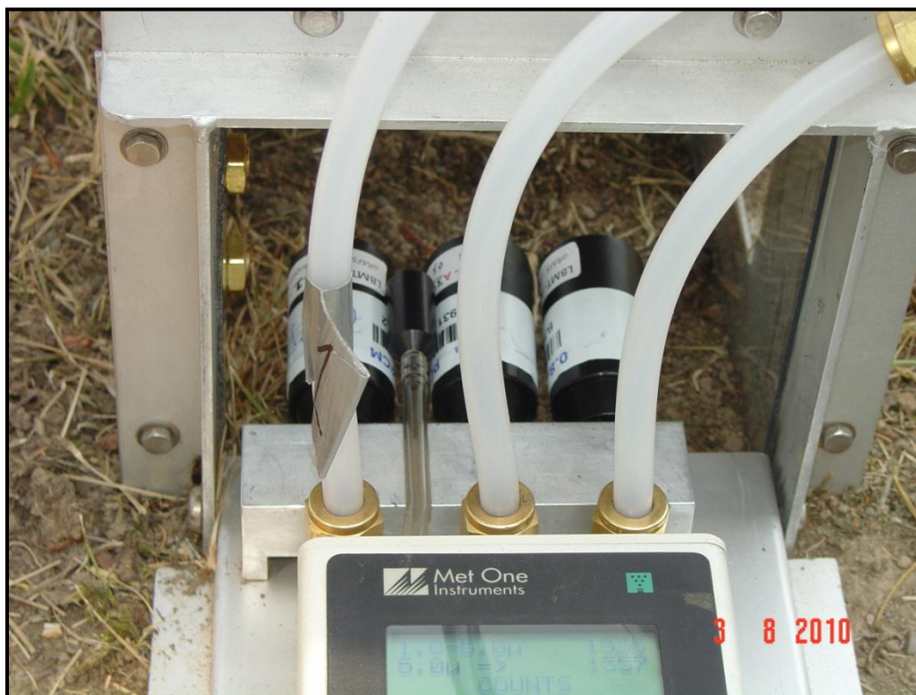
Figure 5. Filter cassette mounting holder and optical particle counter platform at tunnel exit.
