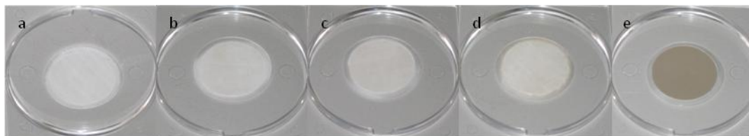
Figure 15. Photographs of 25 mm dia. 0.8 µm pore MCE filters to assess proper loading of particles for direct-transfer TEM analysis. a) unused filter, b) lightly loaded filter, c) ideal, properly loaded filter, d) overloaded filter, e) very overloaded filter.
