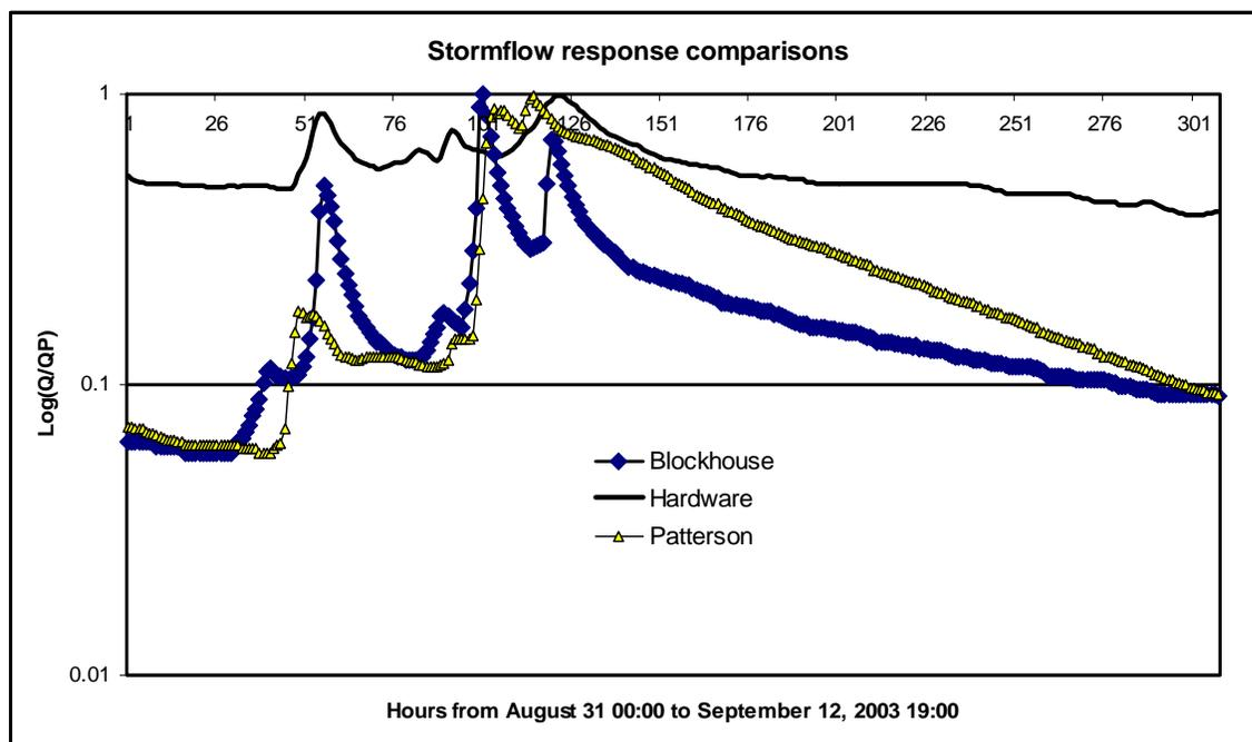
Figure 18. Comparisons of Standardized Hourly Runoff Hydrographs
