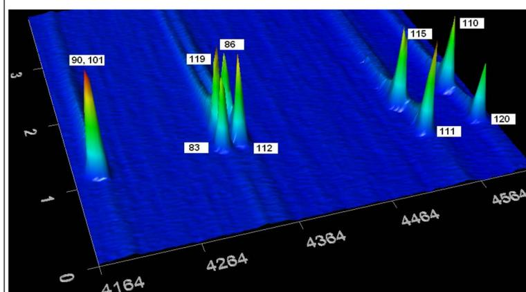
Surface view showing the use of GCxGC-TOFMS in the separation of four pairs of polychlorinated biphenyl isomers with IUPAC numbers beginning from the right of (110 + 120), (115 + 111), (86 + 112), and (119 + 83). The PCB isomers (left pair) numbers (90 + 101), were inseparable under the chromatographic conditions used. However they exhibited different ortho effects (42% and 29% respectively).
