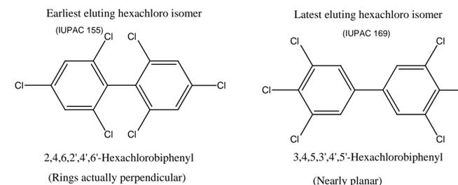
Within the hexachlorobiphenyl congener series, there are 42 hexachlorobiphenyl isomers. Elution time of the hexachlorobiphenyl isomers increased as the number of ortho chlorines decreased. The 246:246 Hexachloro (4 ortho chlorine substitution) was observed to elute the GC column first, while the 345:345 Hexachloro (no ortho chlorine substitution) eluted last.
