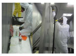
include decontamination of buildings, equipment, and outdoor areas. In support of this role, the EPA's National Homeland Security Research Center (NHSRC) evaluated the performance of nine chemical-based decontamination technologies for their ability to remove Cesium-137 from the surface of unpainted concrete. In addition, NHSRC evaluated various deployment-related characteristics of the products.
