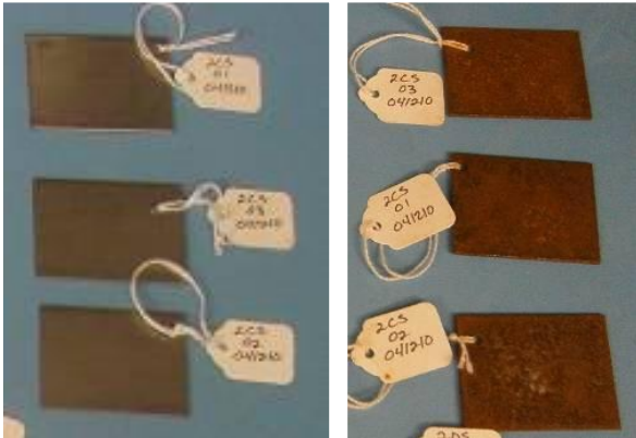
Figure 9. Low carbon steel before (left) and after (right) fumigation showing significant corrosion.
