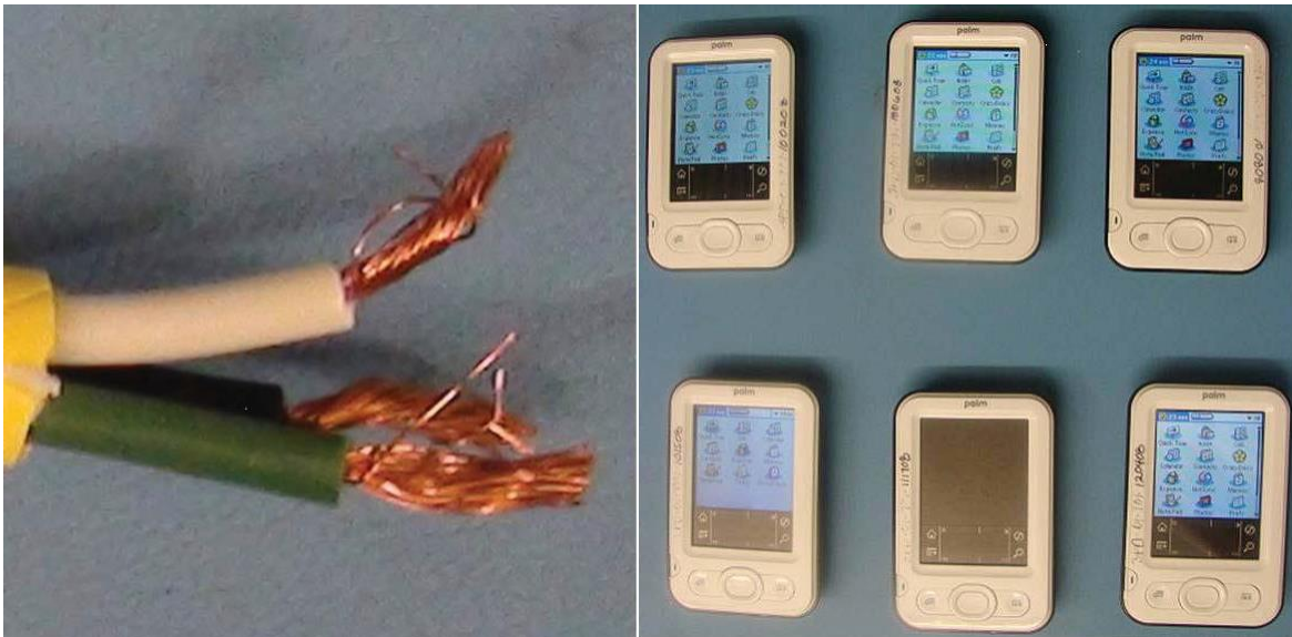
Figure 7. Exposed stranded wire and PDAs powered 12 months after H 2 O 2 gas exposure.
