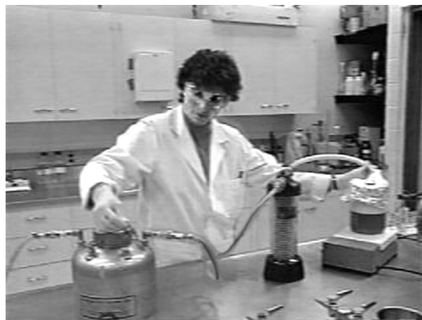
Figure 5. Elution of an electropositive filter with beef extract
