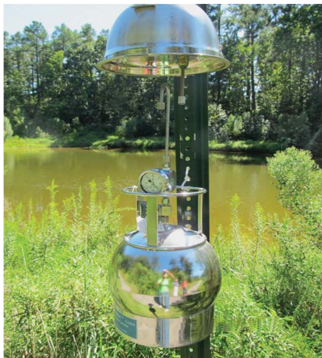
Passive Sampling device
