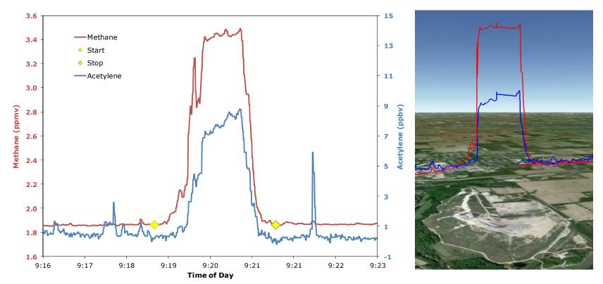
Work with Picarro Inc. to develop and test a simple approach for TC work. A single CRDS instrument to measure methane and acetylene and record meteorological and GPS location data.
