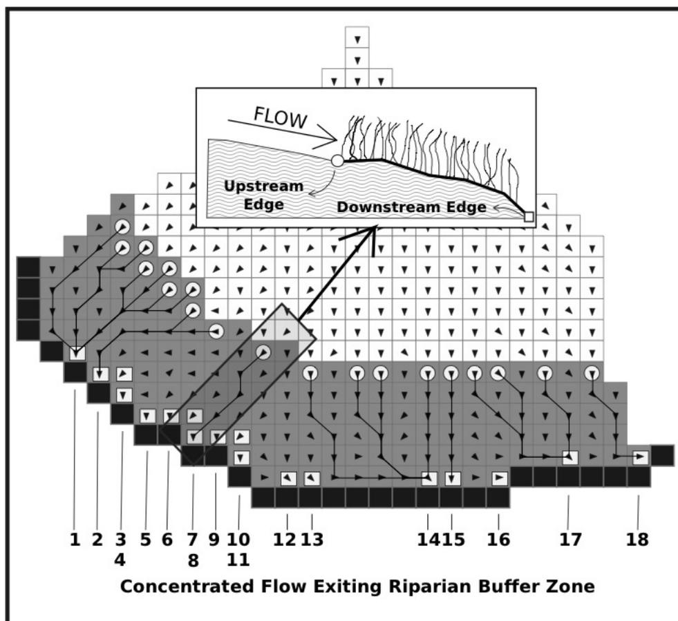
**Figure 3.** GIS characterization of riparian zones. Black lines passing through the buffer zone represent concentrated flow paths (simulated as one-dimensional profiles) and black raster grid cells represent AnnAGNPS reach locations. Circles represent “upstream edge” raster grid cells indicating flow into the riparian zone and squares represent “downstream edge” raster grid cells indicating flow exiting the riparian zone.
