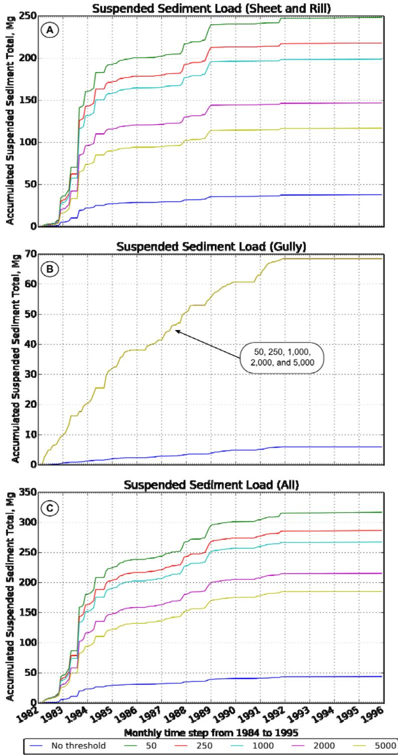
**Figure 14.** Accumulated sediment load downstream of reach 14 generated from sheet and rill (A), ephemeral gullies (B), and all sources (C) for each of the six simulated drainage area thresholds (m<sup>2</sup>) considered.
