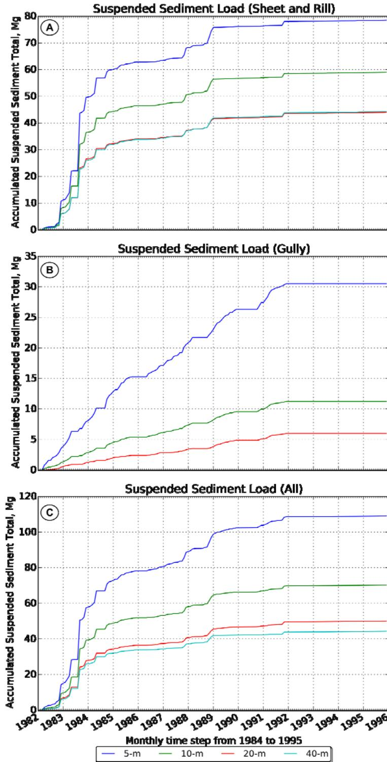
Figure 13. Accumulated sediment load downstream of reach 14 generated from sheet and rill (A), ephemeral gullies (B), and all sources (C) for each of the four simulated buffer width scenarios.
