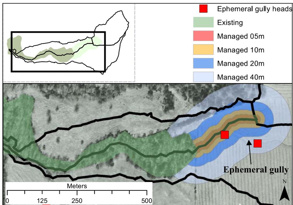
**Figure 9.** Simulated scenarios considered in the evaluation of the riparian buffer width on the AnnAGNPS riparian buffer component estimation of sediment loads.
