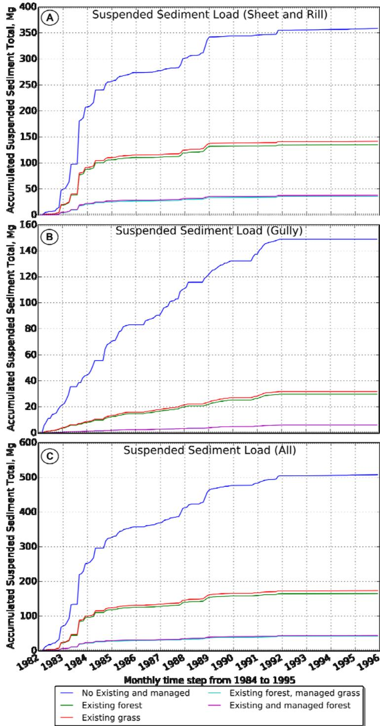
**Figure 12.** Accumulated sediment load downstream of reach 14 generated from sheet and rill (A), ephemeral gully (B), and all combined sources (C) for each of the five simulated vegetation cover type scenarios for the riparian buffer zones.
