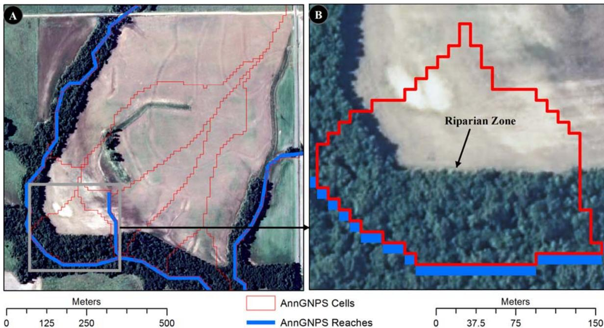
**Figure 1.** Illustration of the AnnAGNPS characterization of the watershed into streams and sub-catchments referred to as AnnAGNPS reaches (blue) and AnnAGNPS cells (red), respectively (A). Existing riparian vegetation zone (edge of field) in each AnnAGNPS cell is identified and characterized for improved calculations of sediment loads (B).
