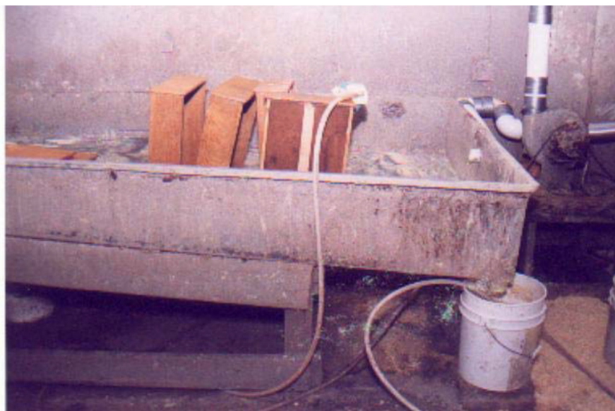
Figure F-1. Typical Flow Tray for Applying Stripper to Furniture
