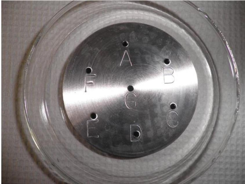
**Figure 2-6. Positive Control Coupon Holder**
