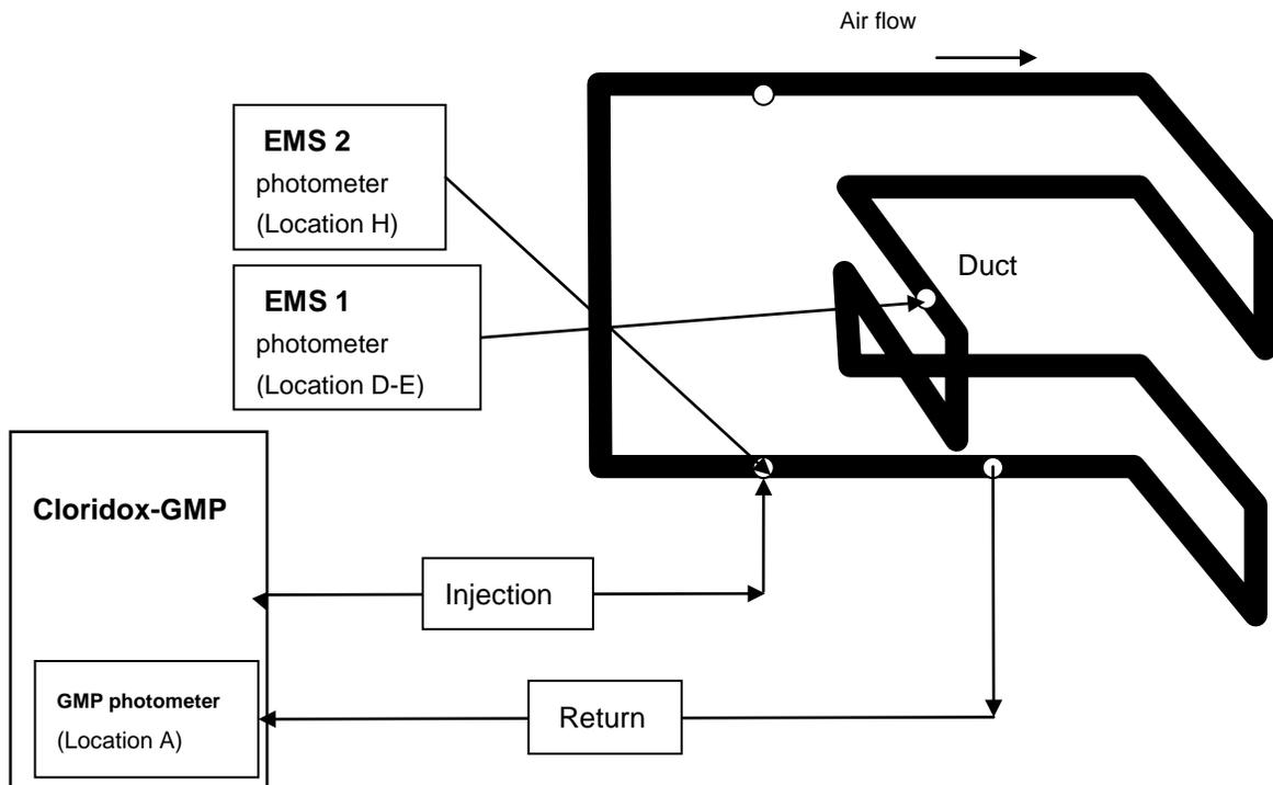
**Figure 2-4. Control Loop Schematic**
