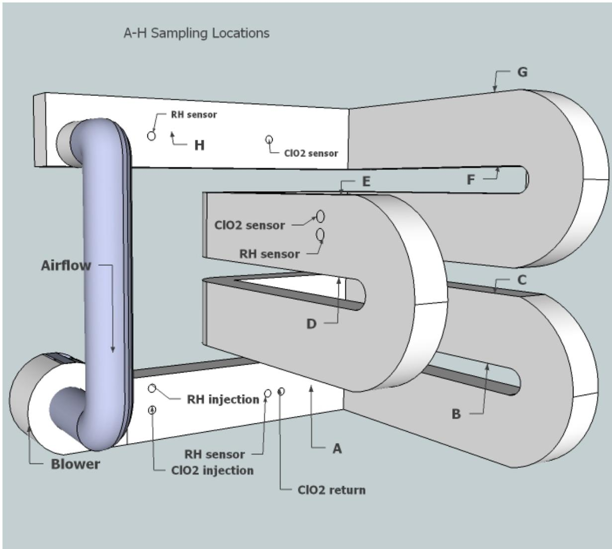
Figure 2-7. Duct Testing Facility ( $\text{ClO}_2$ ) with Sampling and Monitoring Locations Indicated by Letters A-H
