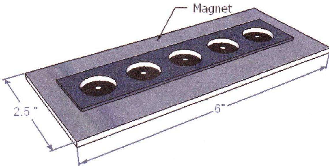
Figure 2-5. Test Coupon Holder Setup
