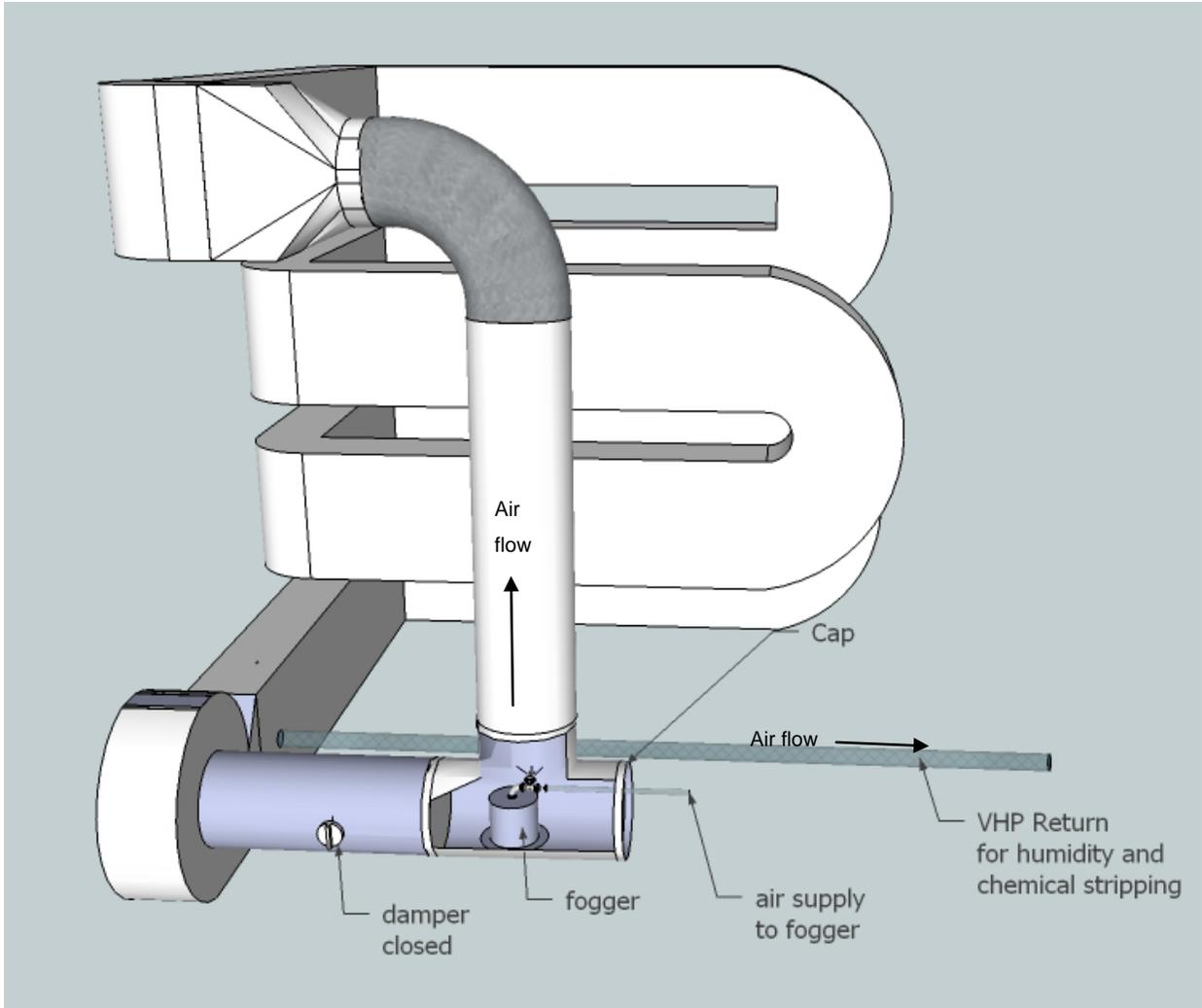
Figure 2-3. HVAC Duct Modification for Fogging Tests
