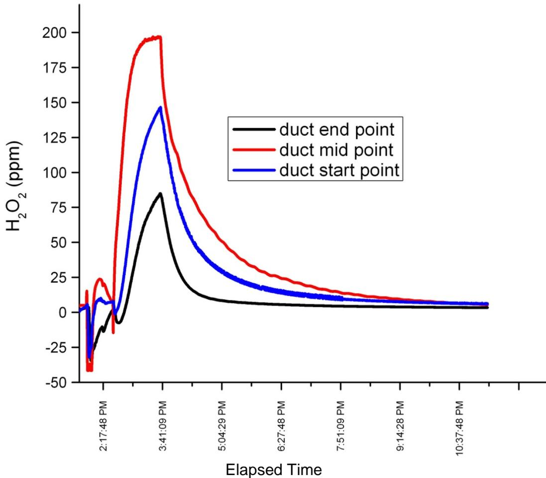
**Figure 3-3. H<sub>2</sub>O<sub>2</sub> Levels During Fogging Test 9**
