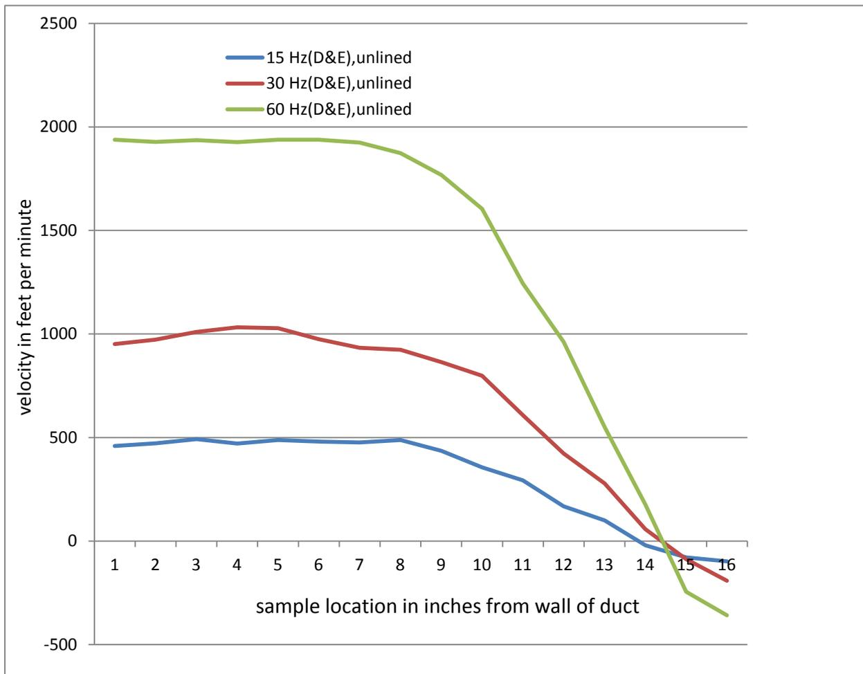
**Figure 3-2. Velocity Traverse Inside the Duct from Location E to D for Unlined Duct.**
