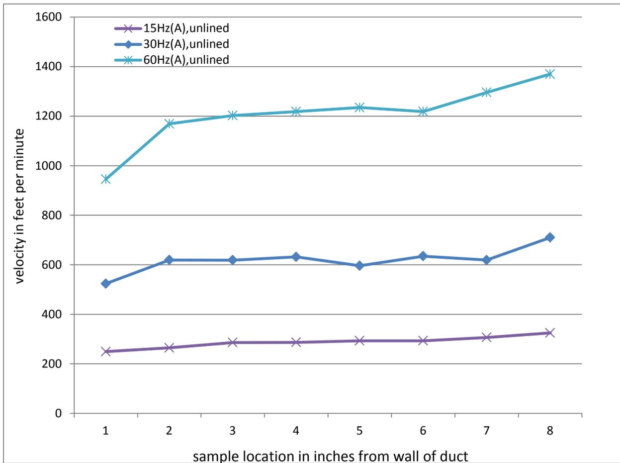
**Figure 3-1. Post-Blower Velocity Traverses Inside Unlined Duct at Point A.**
