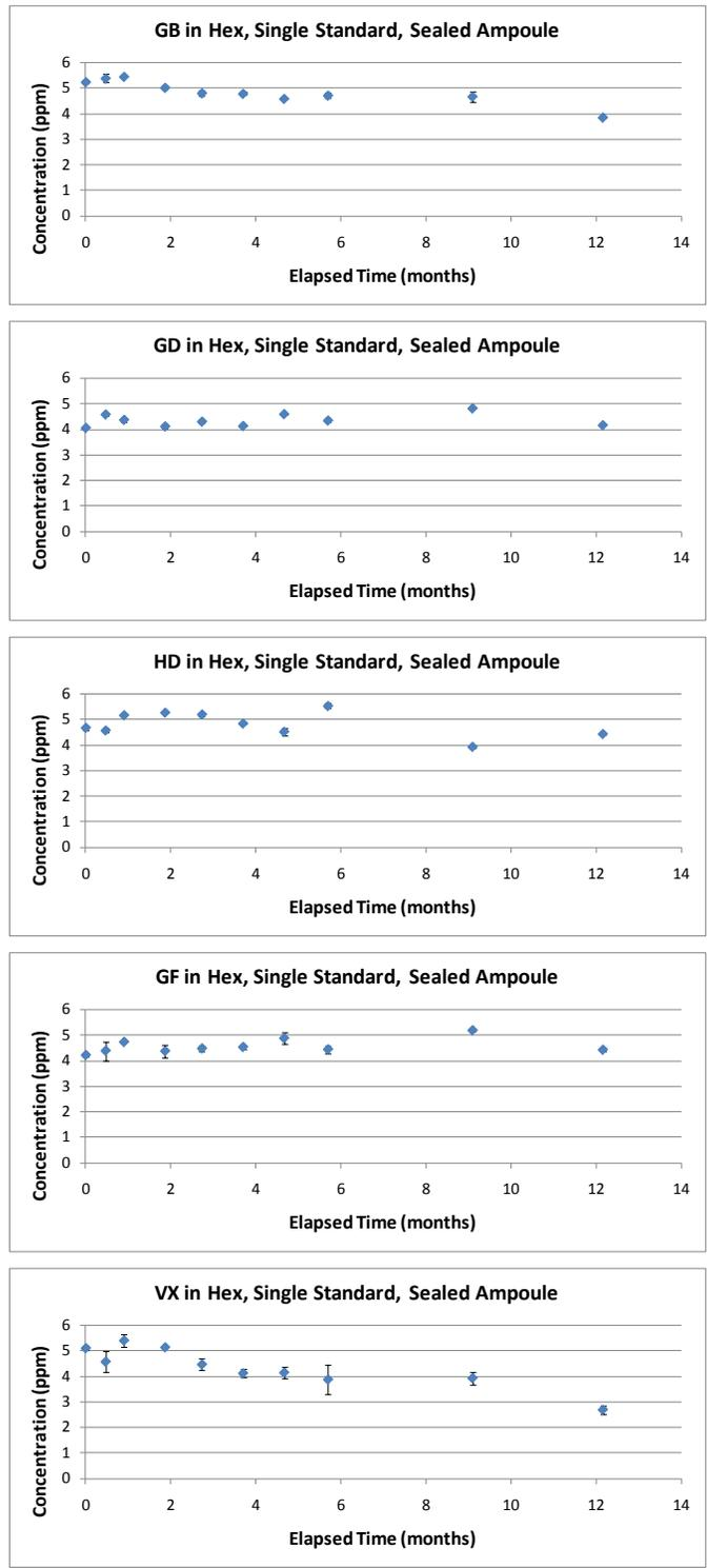
Figure 5. Concentration (ppm) over time (months) for chemical warfare agents present in hexane as a single-component standard in sealed ampoules.
