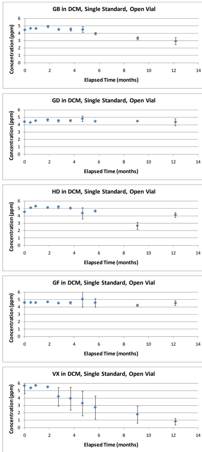
Figure 2. Concentration (ppm) over time (months) for chemical warfare agent single-component standards in dichloromethane in reopened vials
