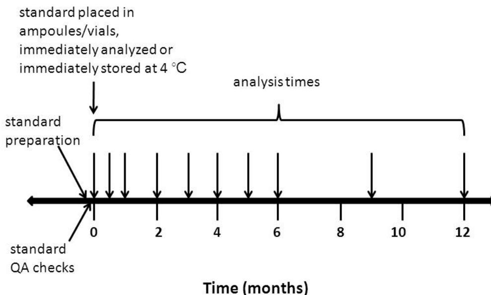
Figure 1. Timeline for standard preparation, ampoulation or ampoulation followed by transfer into a glass vial, and analysis.
