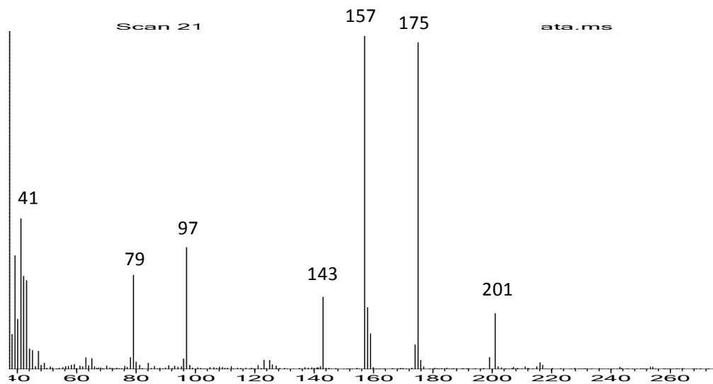
**Diisopropyl dimethylpyrophosphate.** RT = 17.3 min. MW= 258.
