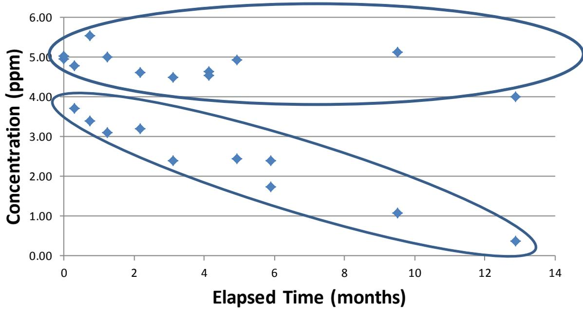
Figure 8. Concentration (ppm) over time (months) for VX in a multiple-component standard in dichloromethane, in sealed ampoules.
