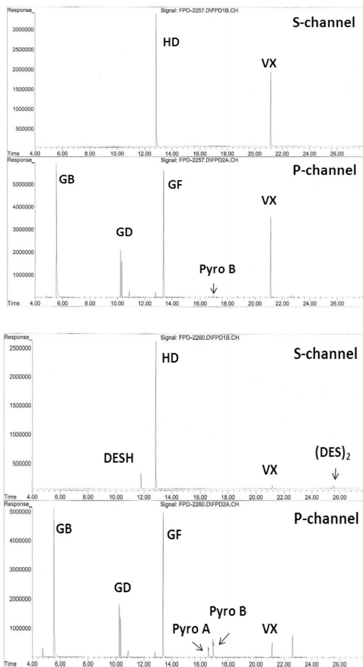
**Figure 12. GC-FPD chromatograms of multiple-component chemical warfare agent standards in dichloromethane after one year of storage, at 4 °C, in a sealed ampoule (top) and in a Teflon-lined, septum-capped vial (bottom).**
