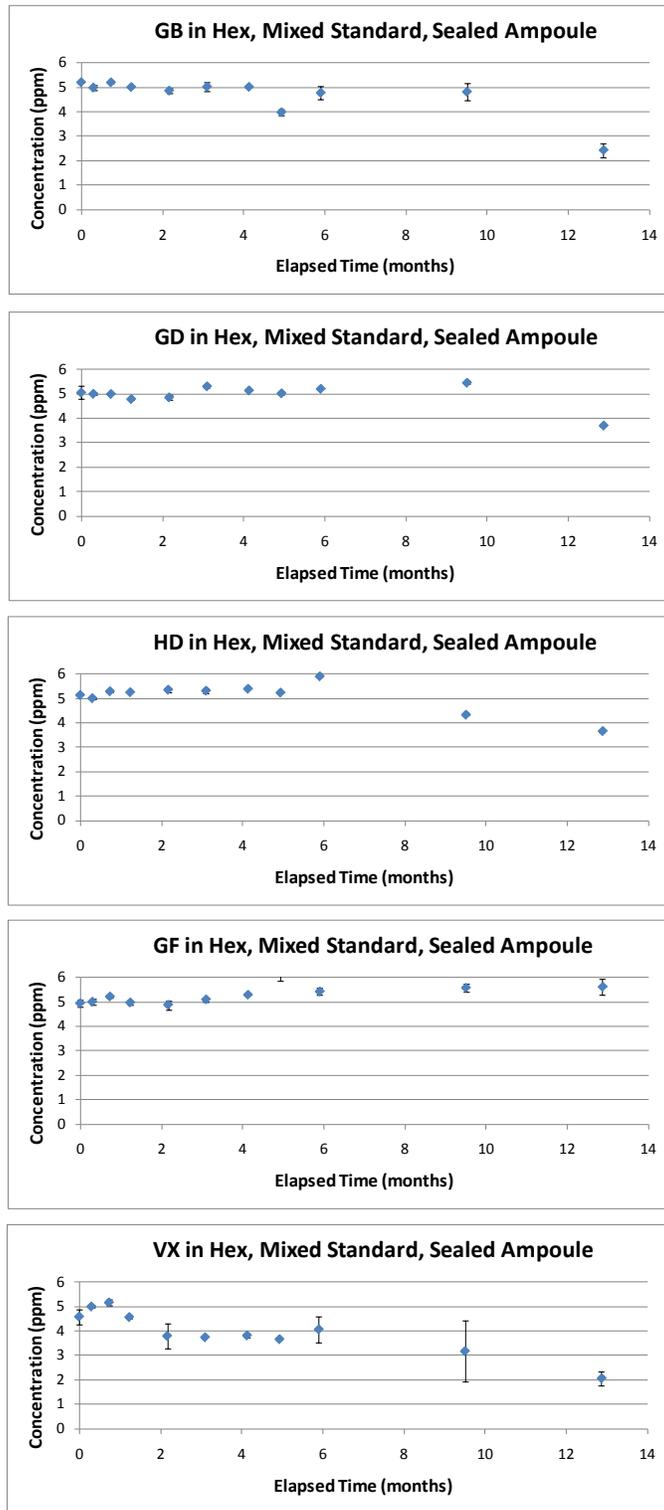
Figure 10. Concentration (ppm) over time (months) for CWAs present in hexane as a multiple-component standard in sealed ampoules.
