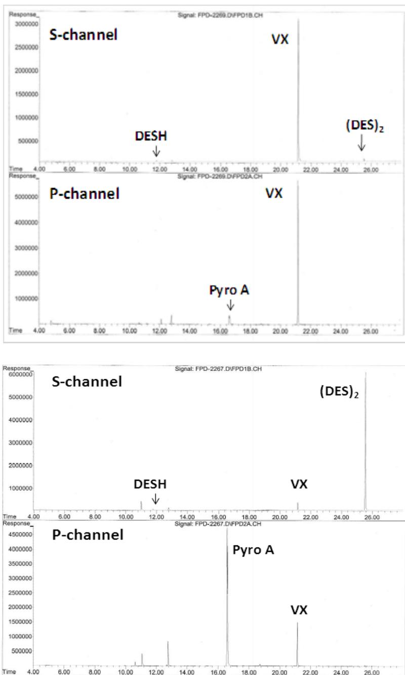
Figure 11. GC-FPD chromatograms (both S and P channels) of single-component VX standards in dichloromethane after one year of storage, at 4 °C, in a sealed ampoule (top) and in a Teflon-lined, septum-capped vial (bottom).
