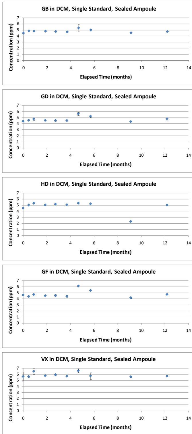
Figure 3. Concentration (ppm) over time (months) for chemical warfare agents in dicloromethane as a single-component standard in sealed ampoules.
