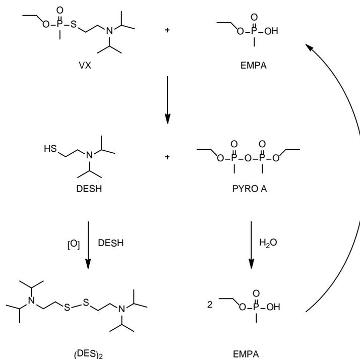
**Scheme 2.** Autocatalytic degradation mechanism for VX initiated by IMPA.
