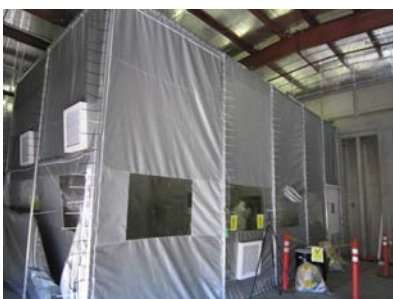
Figure 3-2. Containment tent (outer view) and inner view with test stand containing contaminated coupons.
