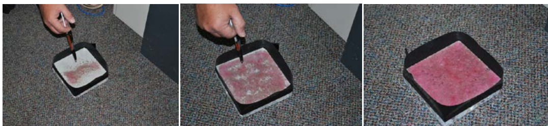
Figure 3-1. Demonstration of contaminant application technique.
