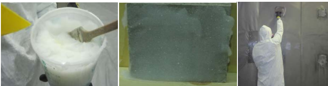
Figure 3-5. ASG before application, as applied to coupon, and during vacuum removal.
