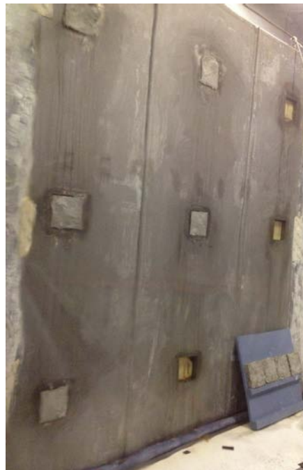
Figure 3-3. Containment tent (outer view) and inner view with test stand containing contaminated coupons.
