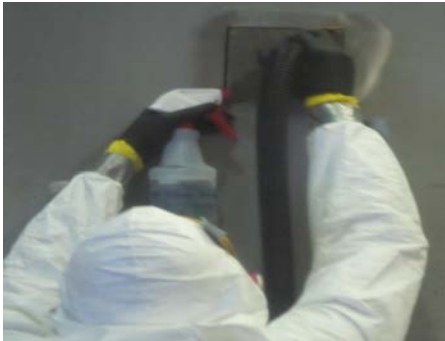
Figure 3-4. Rinsing and vacuuming RRII from concrete coupon
