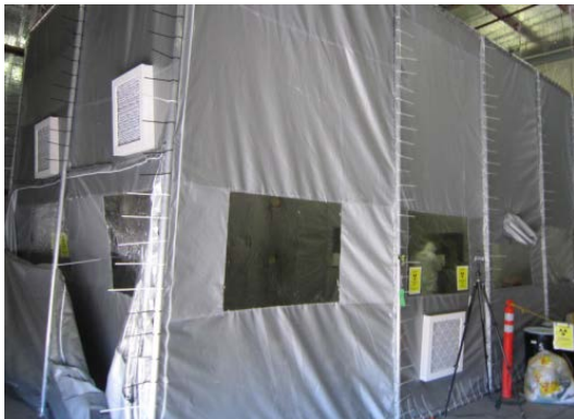
Figure 3-3. Containment tent (outer view) and inner view with test stand containing contaminated coupons.
