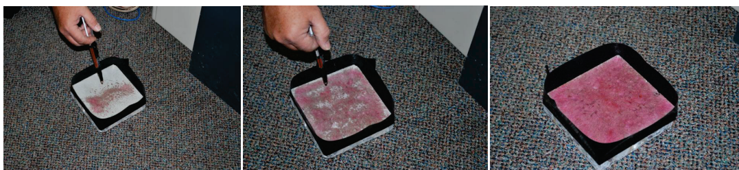
Figure 3-1. Demonstration of contaminant application technique.
