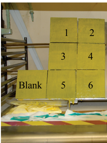
Figure 3-2. Test stand with concrete coupons.
