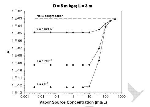
Figure 4. Vapor Intrusion Attenuation Factors Predicted by Abreu and Johnson (2005) Three Dimensional Model as a Function of Separation Distance below Foundation and First Order Biodegradation Rate for a Residential House Scenario (from Abreu et al., 2009).
