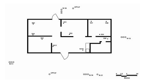
Figure 2. Layout of Office Building and Sampling Locations (scale in metres).
