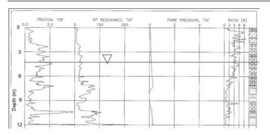
Figure 7. Cone-Penetrometer Log for CPT-LIF-2 Showing Inferred Geology.
