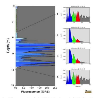
Figure 8. Laser-Induced Fluorescence Log for CPT-LIF-2 showing residual LNAPL in 6.1 to 11.3 m bgs interval.
