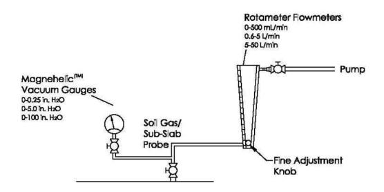
Figure 4. Schematic diagram of pneumatic testing apparatus.
