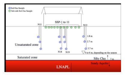
Figure 3. Cross-Section of Office Building and Sampling Locations (schematic) .
