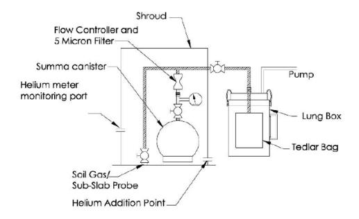
Figure 5. Soil Gas Sample Collection Apparatus.
