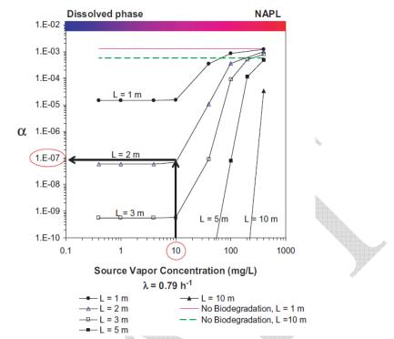
Figure 2. Vapor Intrusion Attenuation Factors Predicted by Abreu and Johnson (2005) Three-Dimensional Model for a Range of Source Total Hydrocarbon (benzene) Vapor Concentrations and Separation Distances for a Residential House Scenario (from Abreu et al., 2009).
