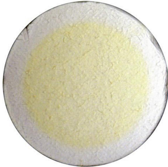
**Figure 4.** Isokinetic sampler filter showing collected uranine-tagged particles.
