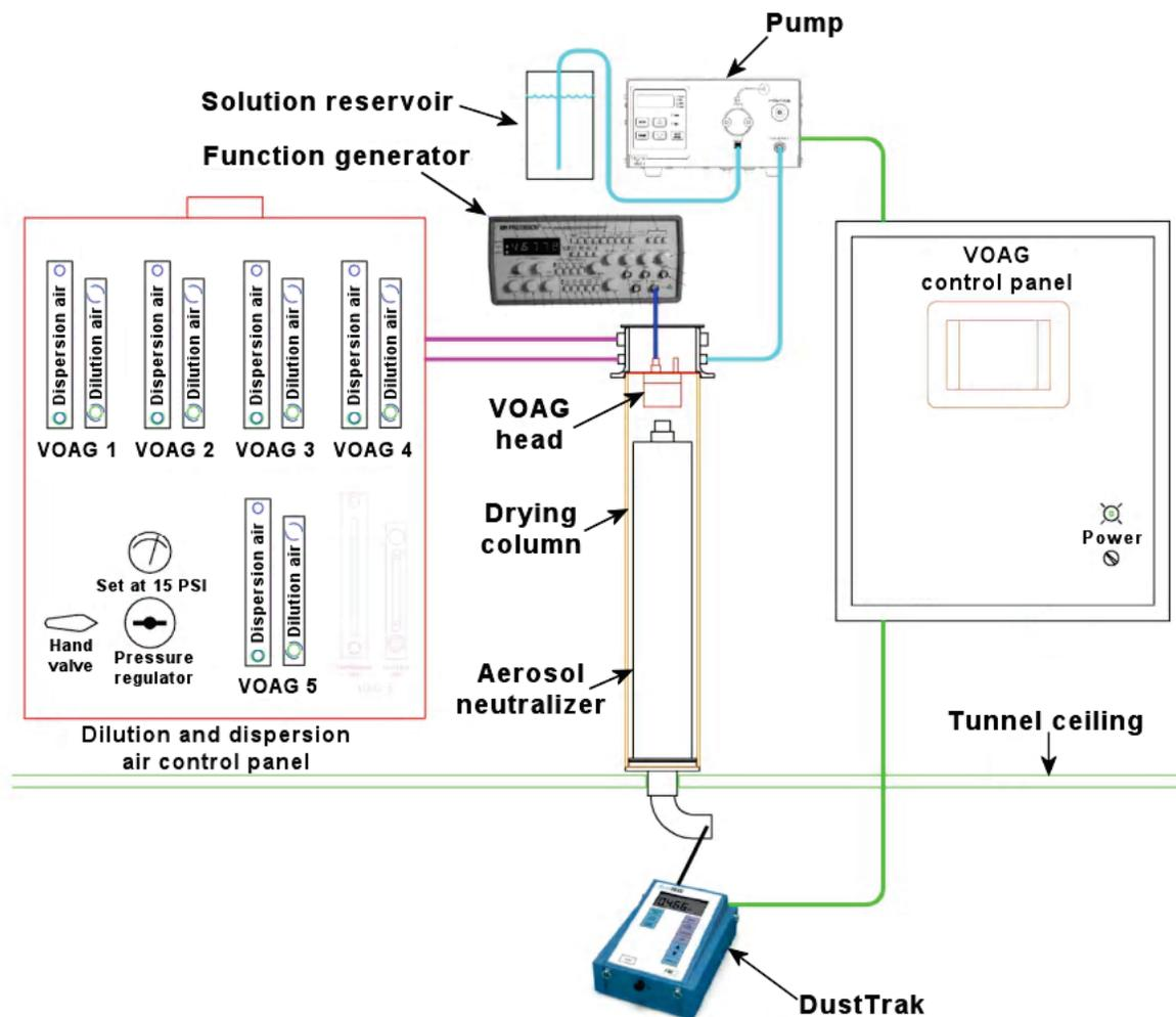
Figure 2. Aerosol generation system
