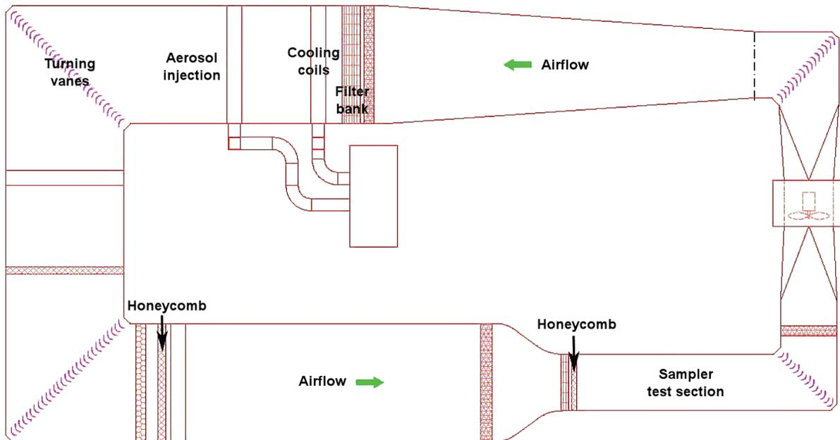
Figure 1. Plan view of the EPA NHSRC aerosol wind tunnel.
