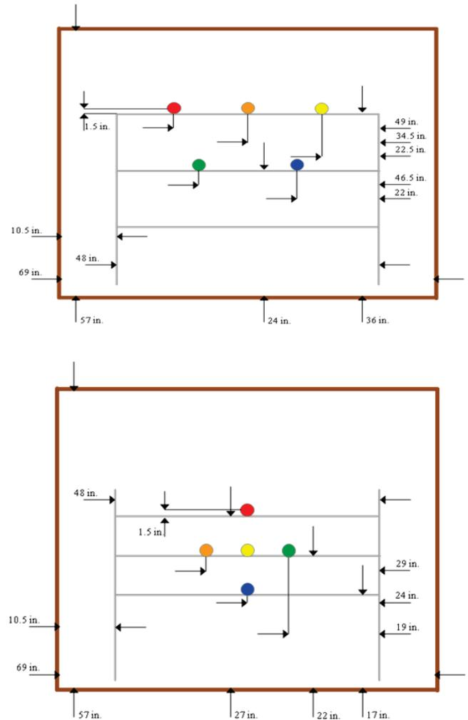
**Figure 3.** Critical dimensions of rake samplers showing locations of aerosol sampling points for two configuration.
