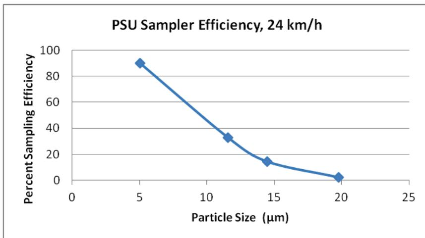
**Figure 5.** PSU sampler efficiency data plotted against particle size for all three test wind speeds.
