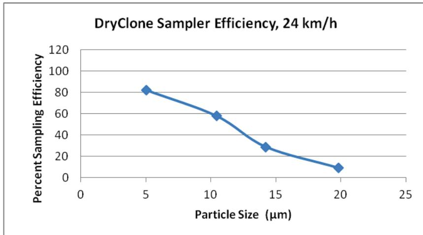
Figure 6. DryClone™ sampler efficiency data plotted against particle size for all three test wind speeds.
