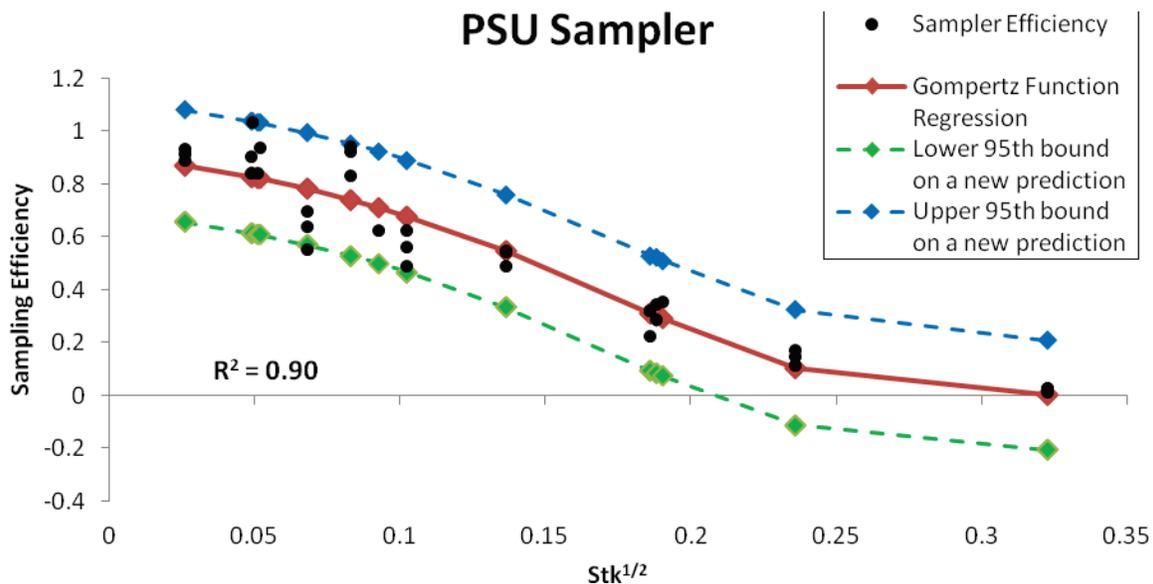
**Figure 7.** PSU sampling efficiency plotted as a function of the square root of  $Stk$ . Regression lines are the Gompertz functions with values of  $a$ ,  $b$ , and  $c$  from Table 5.
