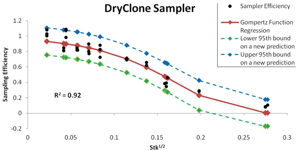
**Figure 8.** DryClone™ sampling efficiency plotted as a function of the square root of  $Stk$ . Regression lines are the Gompertz functions with values of  $a$ ,  $b$ , and  $c$  from Table 6.
