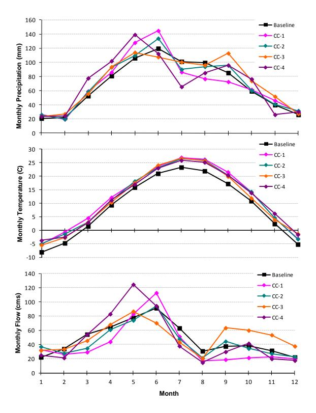
Figure 3-6. Mean monthly precipitation (mm), temperature (°C), and streamflow (cms) for the NARCCAP-derived climate change scenarios, CC-1, CC-2, CC-3, CC-4, and the baseline scenario.
