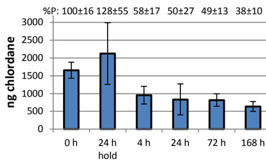
**Figure 1. Persistence evaluation - percent persistence and chlordane remaining on cement (left) and backing (right)**
