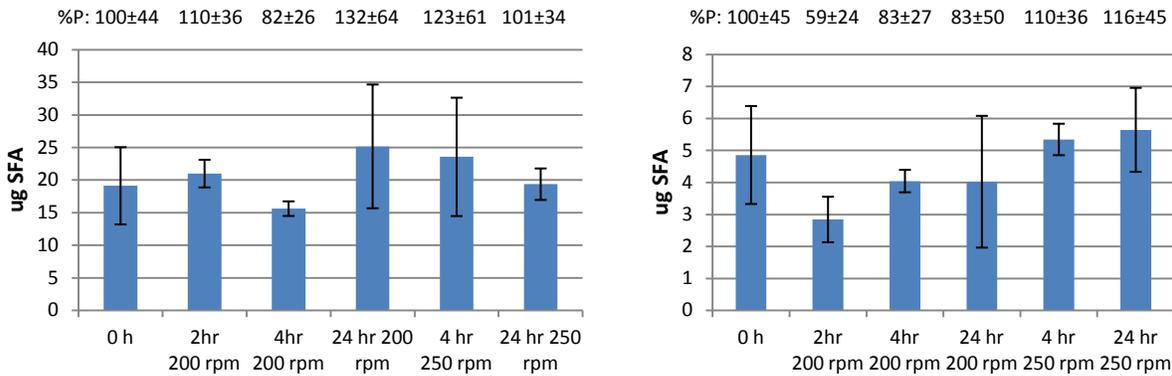
**Figure 8. Flushing evaluation - percent persistence and SFA remaining on cement (left) and backing (right).**
