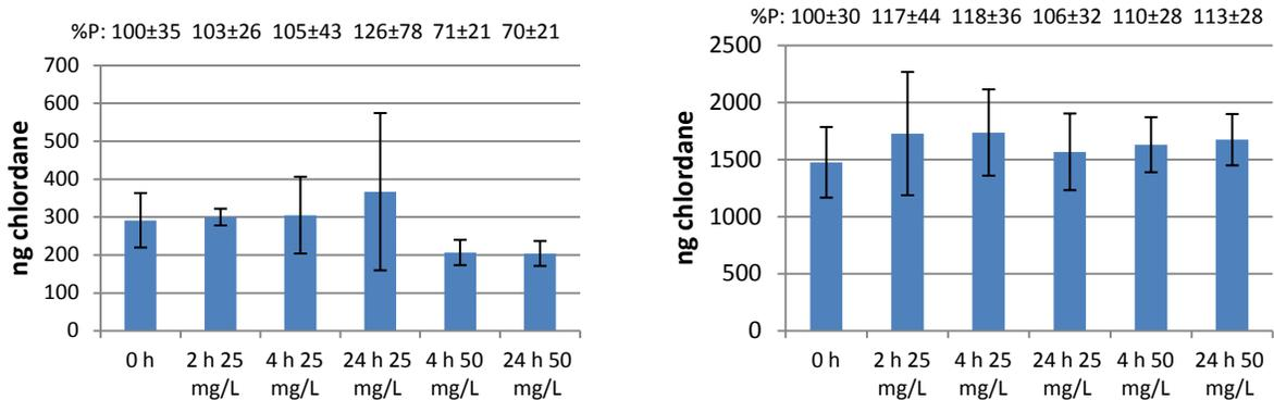
**Figure 3. Hyperchlorination evaluation - percent persistence and chlordane remaining on cement (left) and backing (right)**
