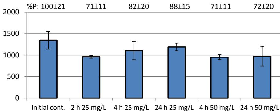
**Figure 6. Hyperchlorination evaluation - percent persistence and chlordane remaining on PVC**
