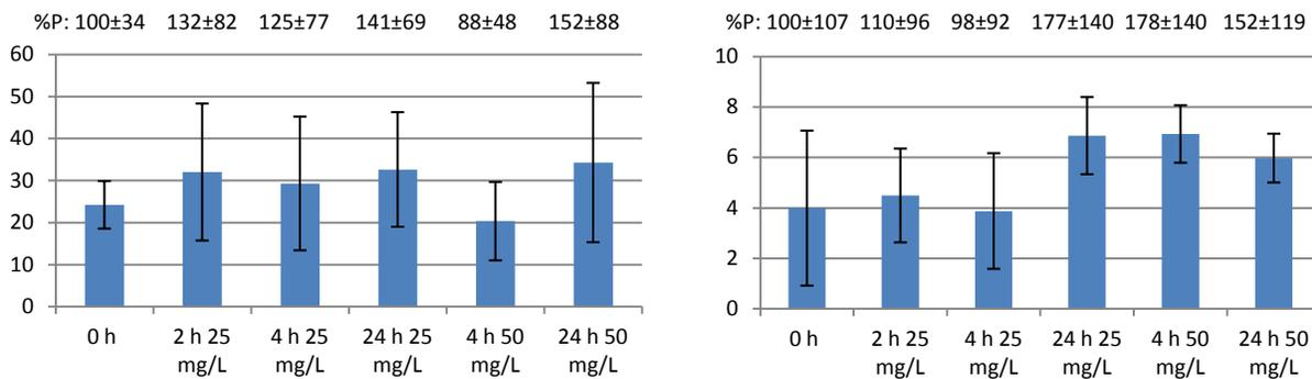
**Figure 9. Hyperchlorination evaluation - percent persistence and SFA remaining on cement (left) and backing (right)**
