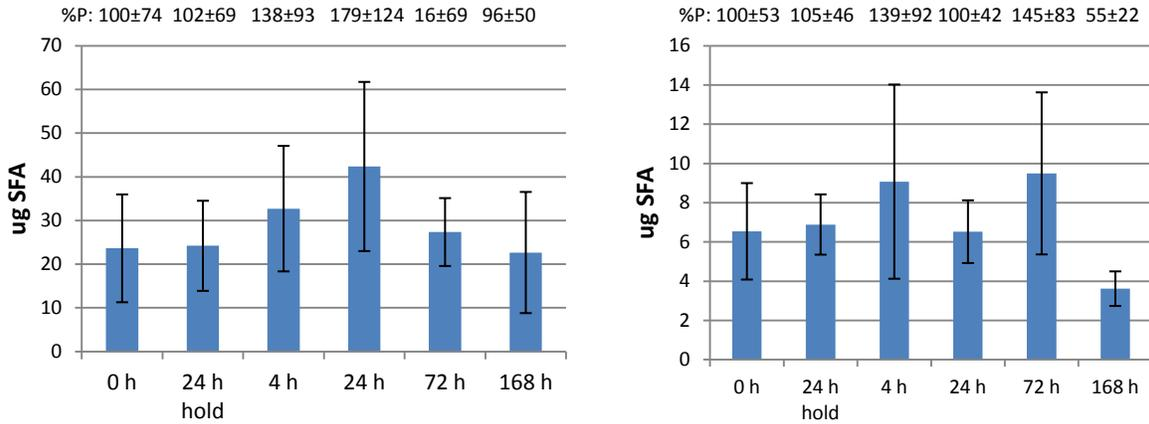
**Figure 7. Persistence evaluation - percent persistence and SFA remaining on cement (left) and backing (right)**
