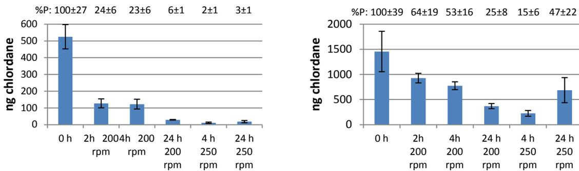
**Figure 2. Flushing evaluation - percent persistence and chlordane remaining on cement (left) and backing (right)**
