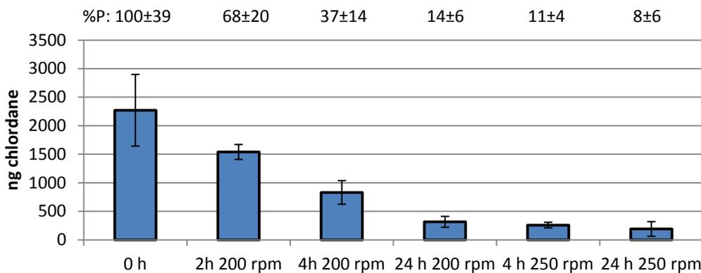
**Figure 5. Flushing evaluation - percent persistence and chlordane remaining on PVC**
