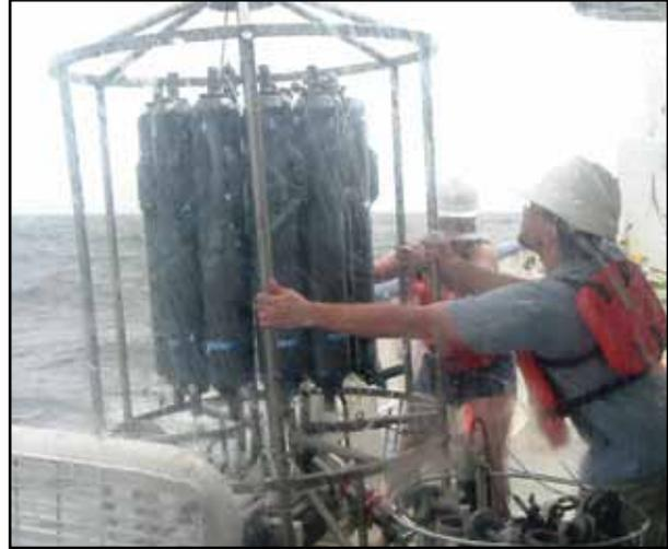
Researchers retrieve the CTD rosette, used for collecting water and measuring dissolved oxygen and other oceanographic parameters, after a sampling profile is completed during rough seas.
