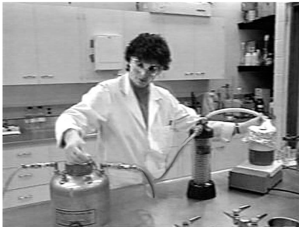
Figure 4. Elution of an electropositive filter with beef extract
