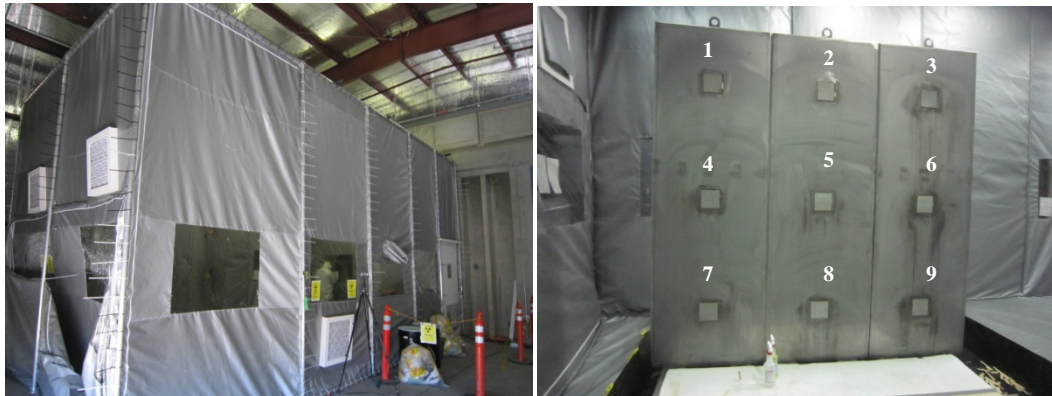
Figure 3-2. Containment tent: outer view (left) and inner view with test stand containing contaminated coupons with numbered coupon positions (right).
