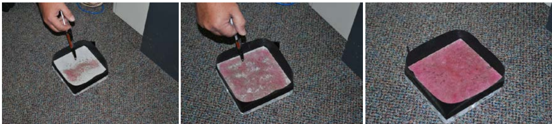
Figure 3-1. Demonstration of contaminant application technique.
