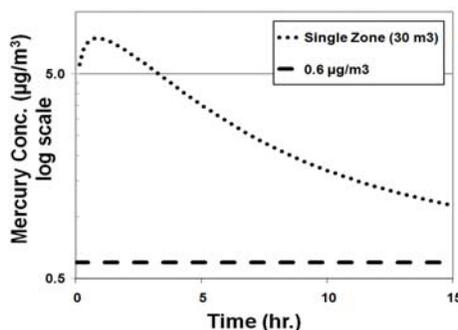
Figure 2: Modelled potential indoor air mercury concentrations following CFL breakage in a single room, compared to the one hour Acute CA-REL (CA.GOV, 2008).
