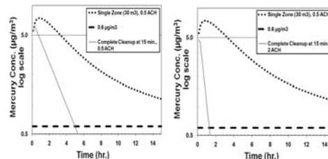
Figure 3a: Using the Aucott emission rate in an example room with 30 m<sup>3</sup>, 0.5 ACH, and full cleanup within 15 minutes, the indoor elemental mercury concentrations in air fall below the California one hour reference value within about five hours.
