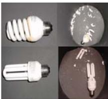
Figure 1b: When the glass tubing of a CFL breaks, elemental mercury is released, necessitating proper cleanup and disposal to minimize indoor mercury emissions and concentrations in air.
