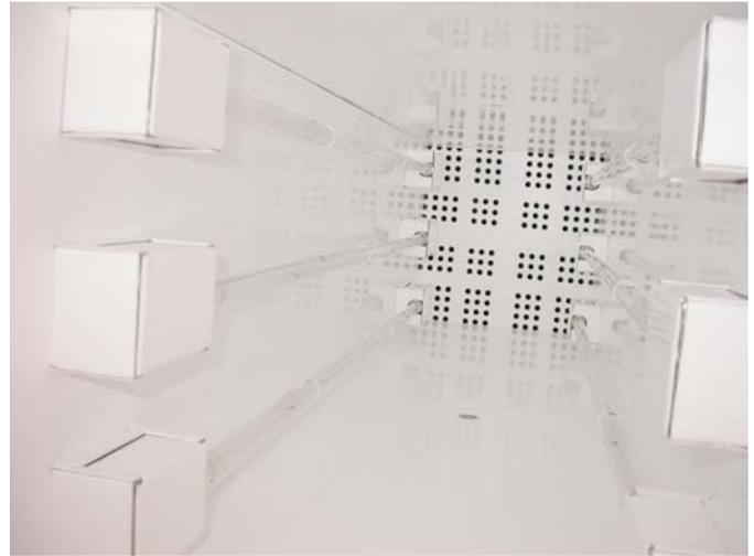
Figure 2-2. Device installed inside the test rig. There are 6 lamps.
