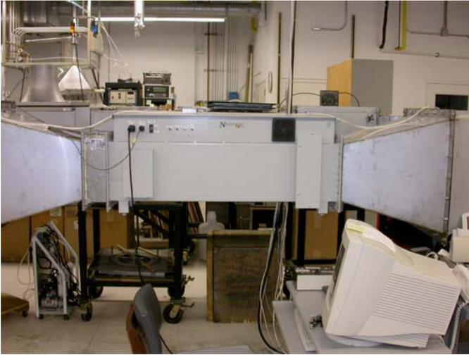
Figure 2-1. BioProtector BP114i installed in the test rig. The ballast boxes are on the top of the device.
