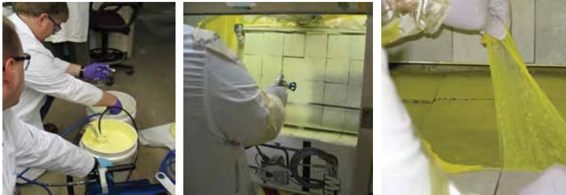
Figure 2-1. Preparation (left), Application (middle), and Removal of Stripcoat (right)
