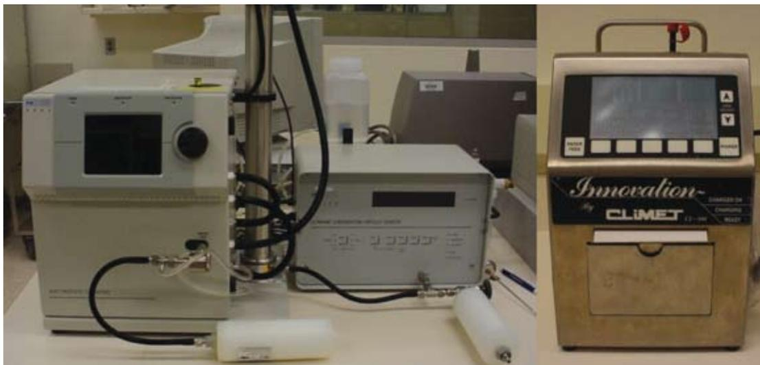
**Figure 4.** Aerosol Sampling Instruments, TSI SMPS (left) and Climet CI-500 (right)
