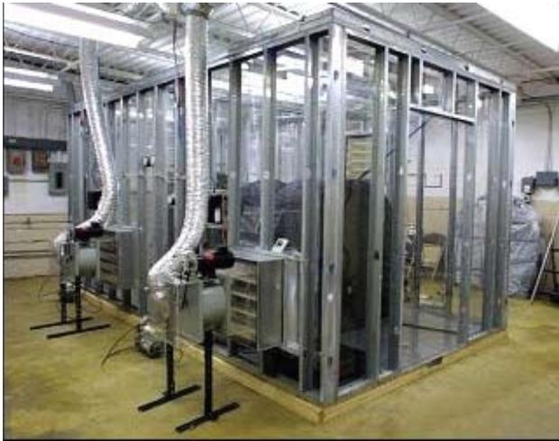
**Figure 15.** Test Chamber for In-Room Experiments
