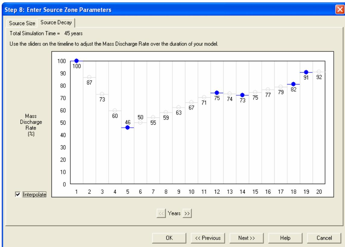
**FIGURE 3. Input screen for entering variable source loading over time for Bioplume 4**
