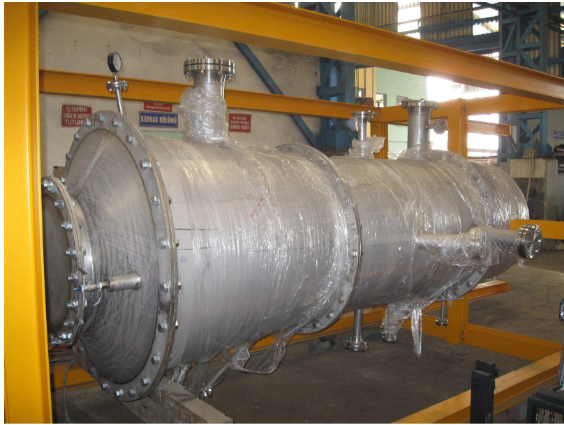
Figure 2 Gasifier Schematic and Completed Main Assembly
