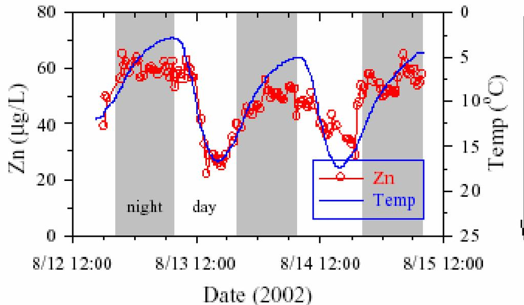
Figure 11. Diel variation in zinc concentrations and temperature in Fisher Creek, MT measured *in situ* with the Zn-DigiScanner. Submersible autoanalyzers such as this are beginning to provide fine-scale temporal and spatial data that was previously unattainable to aquatic chemists. Data of T. Chapin and R.B. Wanty.
