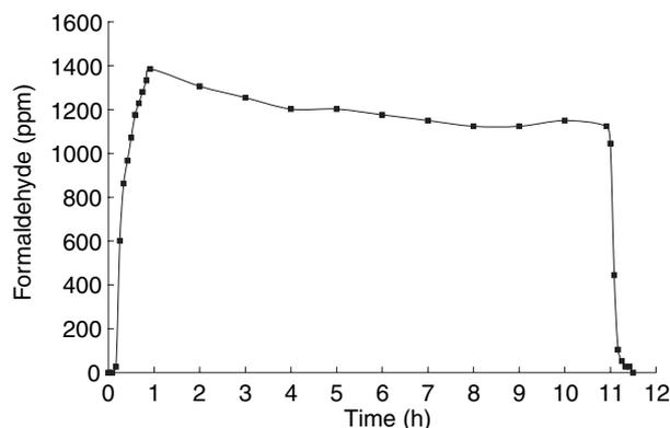
**Figure 1** Formaldehyde concentration measured inside the glove box. This figure represents the data collected for a single decontamination run from the start of gassing through neutralization. During the decontamination runs, the temperature ranged from 22–23°C and the relative humidity ranged from 70–75%.
