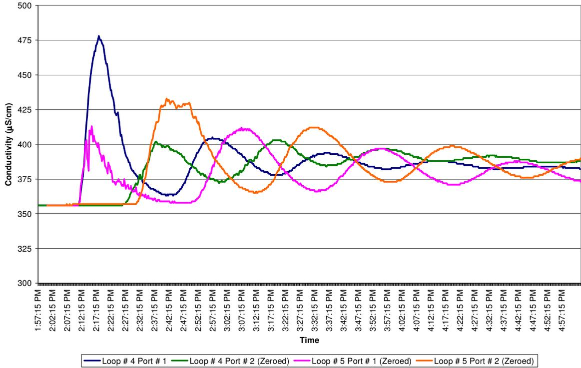
**Figure 5. 3 gpm Tracer Run - 3 Min Injection**
