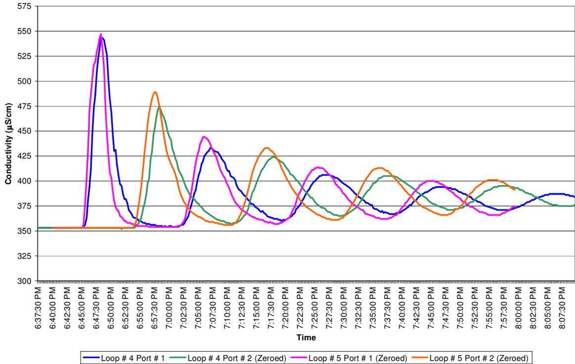
**Figure 6. 6 gpm Tracer Run - 3 Min Injection**
