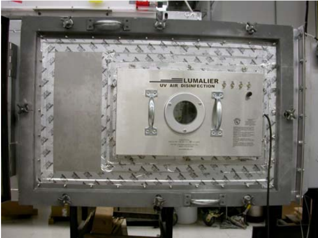
Figure 2-1. Ballast enclosure installed on The outside of the test rig.
