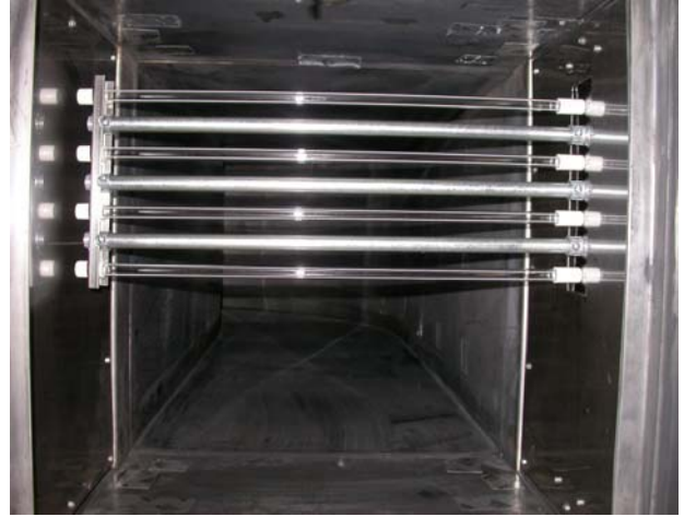
Figure 2-2. Device installed inside the test rig. There are 4 lamps and 3 support rods.
