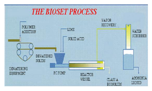
Significant heat is produced as calcium oxide, quicklime, is added at a level of 40-50% dry weight to dewatered sludge. The calcium hydroxide, produced from this reaction, reacts with the sulfamic acid to produce even more heat. Since the calcium oxide to sulfamic acid ratio is approximately 100:1, the pH of
