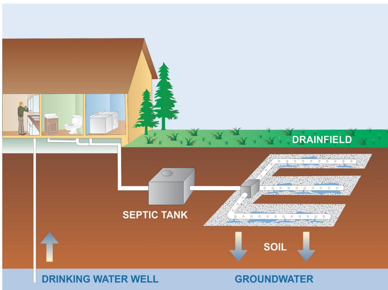
**Figure 3.14** Schematic of a residential septic system (Credit: Snohomish County, WA)
