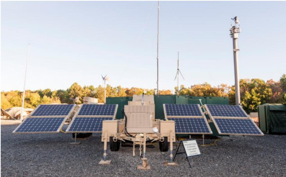
**Figure 3.8** REDUCE mobile solar panels developed for generating electrical power at forward U.S. Army base camps (Credit: U.S. Army photo)
