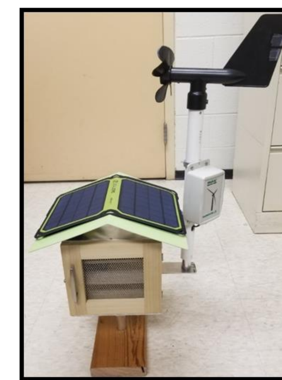
Figure 8. Solar Powered Air Quality Bird House (S-PAQ) includes solar-powered fixed system. Black Carbon Aethlabs AE-51 sensor, NO 2 CairClip sensor, and wind speed/direction sensor.
