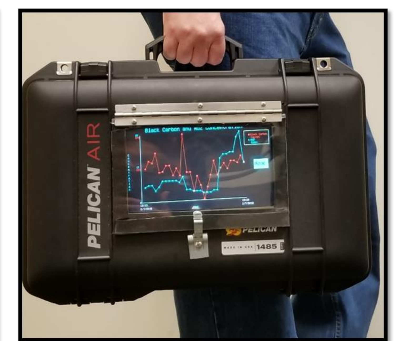
Figure 9. Portable Air Quality Sampler (PAQS) is an Arduino-based portable system with GPS, Black Carbon Aethlabs MA-200 sensor, NO 2 CairClip sensor, and interactive display with RETIGO-ready files.
