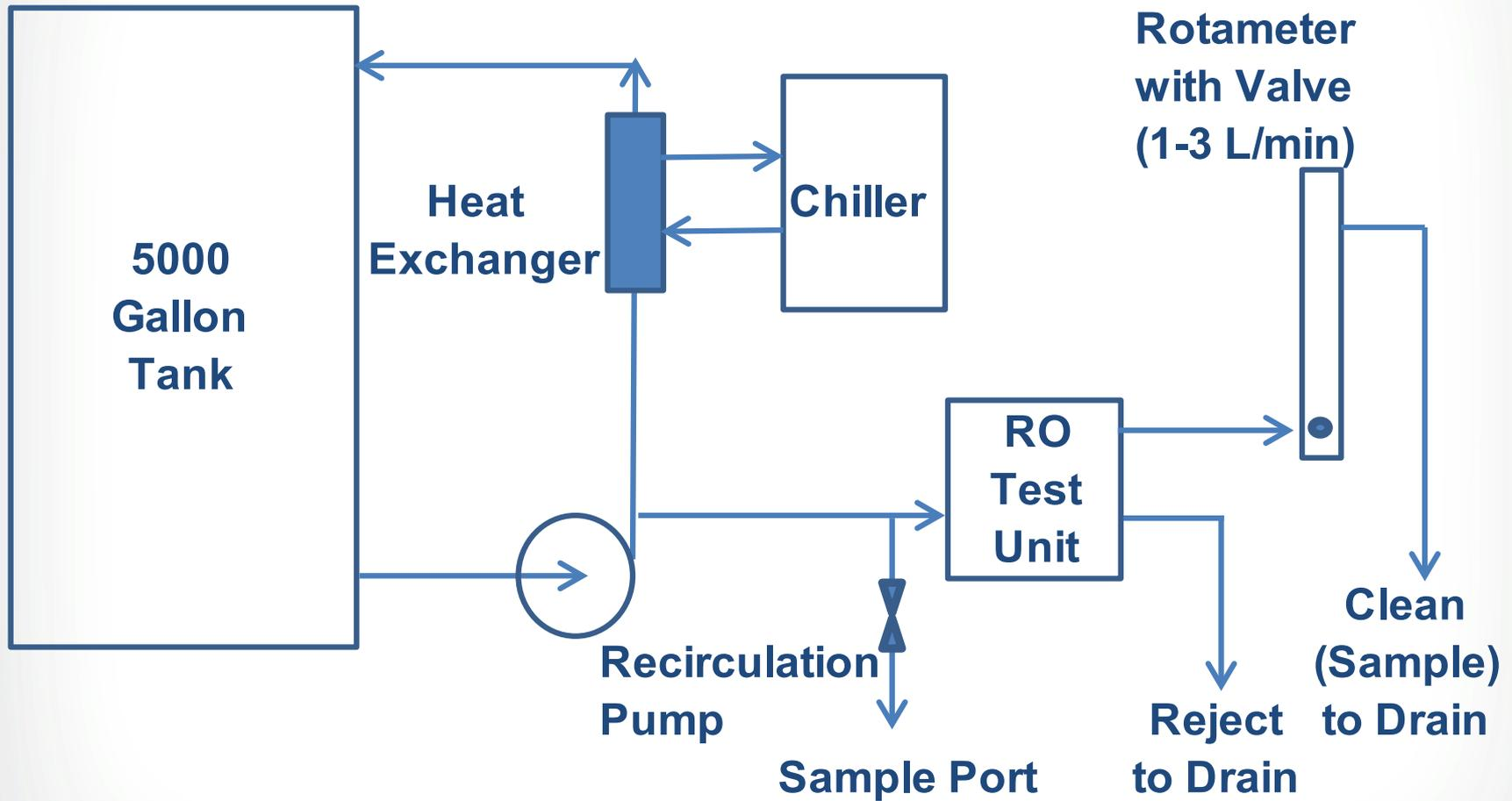
Sample Ports – Influent from 5000 gallon tank line and Effluent from RO permeate line.
