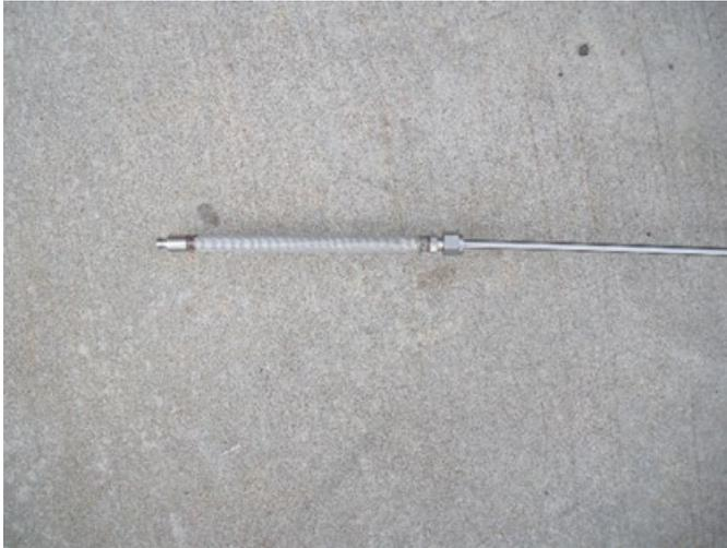
**Figure 8.** Photograph of stainless-steel screen and tubing used for probe construction.
