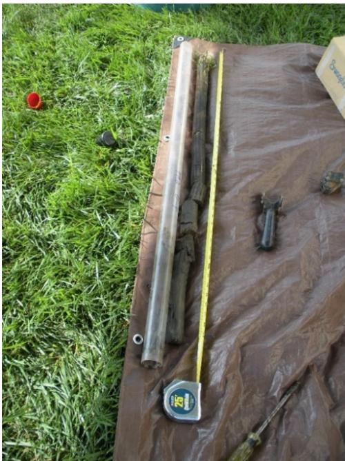
**Figure 4.** Photograph of soil core removed from clear PVC liner.
