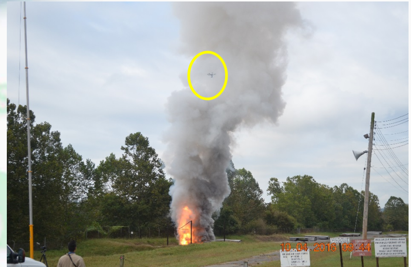
UAV/Kolibri sampling OB plume at Radford AAP
