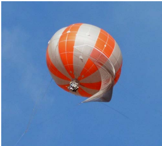
Figure 2-9. Aerostat with the Flyer instrument sampling package.
