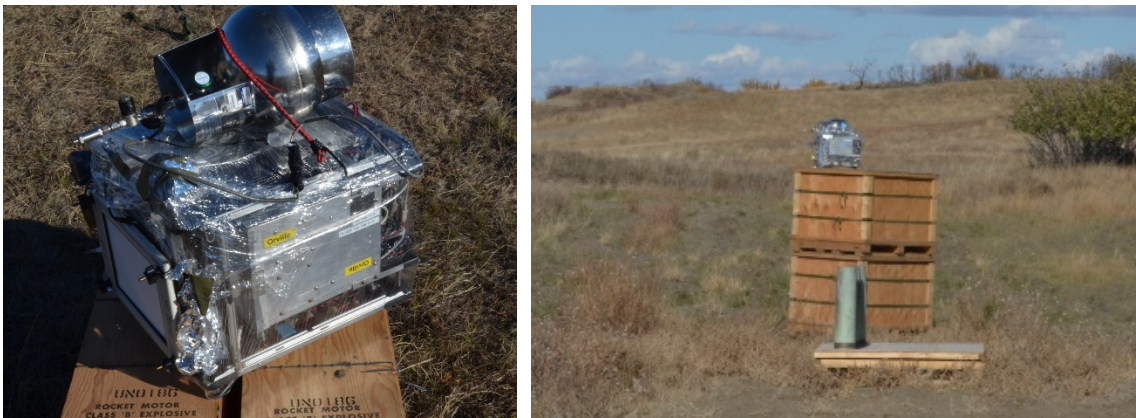
Figure 2-7. Ground based sampling for HC smoke grenade (left), and Red phosphorus (right)
