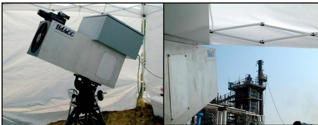
Figure 1. IMACC PFTIR Radiometer.
