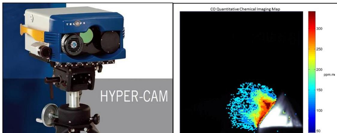
Figure 2. TELOPS Mid-Wave Hyper-Spectral Imager.
