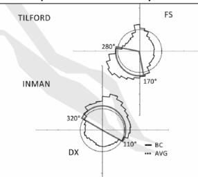
General agreement between mobile and stationary data indicating downwind excess BC / light-absorbing particles
