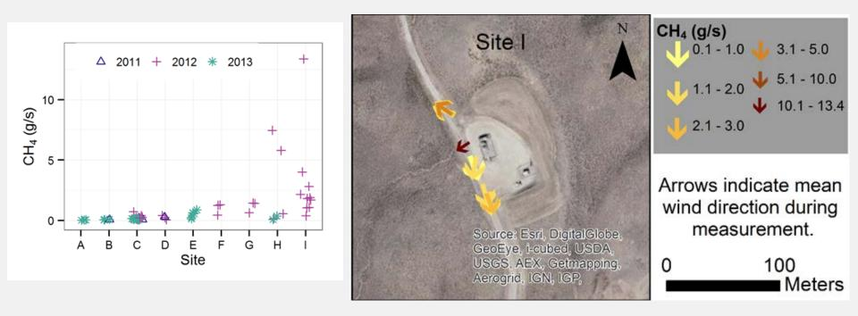
20 min stationary measurements using a mobile platform (SUV) and inverse Gaussian plume dispersion model (OTM 33A)
