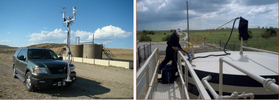
OTM 33A was used to quantify  $CH_4$  emissions remotely at 210 pads in TX, CO, and WY (2010-2013).
