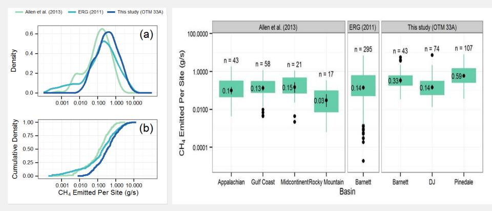
Different measurement techniques capture different aspects of the distribution. Remote measurements useful for locating high emitters.
