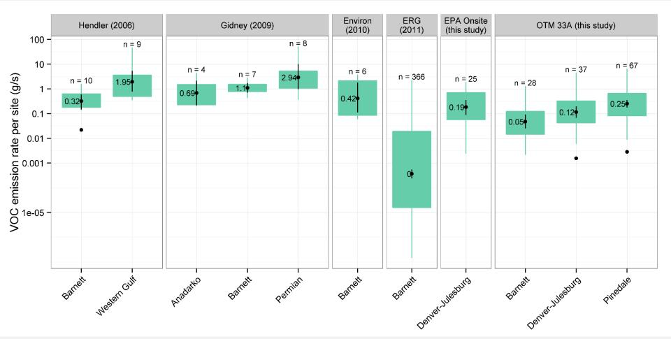
Onsite EPA measurements were similar to remote measurements. ERG (2011) measurements are significantly lower, likely due to choice of compounds used in the canister analysis.
