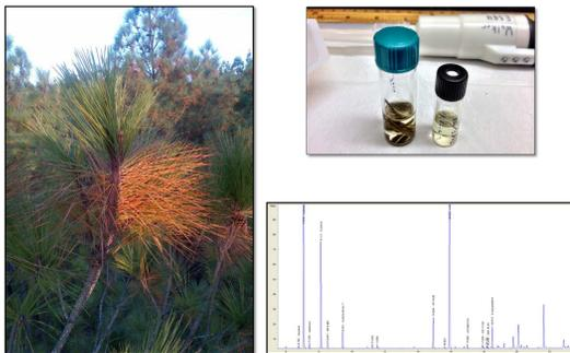
Figure 2: Clockwise from top left: a *P. taeda* branch displaying first and second year needles; solvent extraction process; GC-FID/MS analysis.
