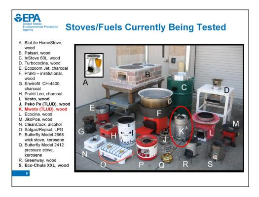
This photo shows stoves we are currently testing. Stoves listed in bold text are batch-fueled with wood. The stove shown inside the red circle is the one we will focus on in this webinar. It is a batch-fueled pyrolytic TLUD (top-lit up-draft) type cookstove. Thanks to Karsten Bechtel and CREEC in Uganda for permission to use preliminary results for the Mwoto stove for discussion purposes today and for review of the spreadsheet.
