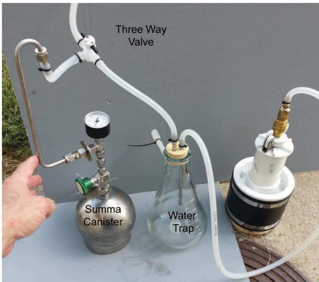
**Figure B.2.** An arrangement of a sampling cap connected to the riser of a well, a water trap and a sampling port connected to a Summa Canister.
